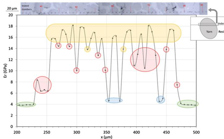
FIGURE IV.16 – Reduced modulus of hemp fiber collected from Ref. [Perrier 16]
