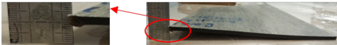
FIGURE III.24 – The deformation of the tested plate during water aging
