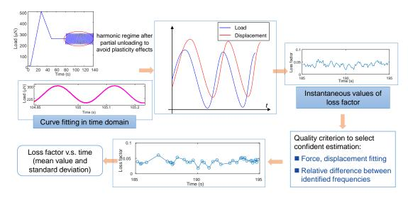
FIGURE IV.6 – Post-processing of the load and displacement for damping identification
