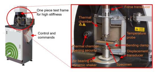
FIGURE II.3 – Main assets in Metravib® DMA+300
