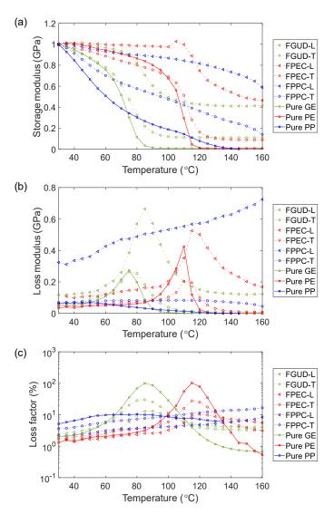
FIGURE II.20 – (a) Normalized storage modulus, (b) loss modulus, (c) loss factor of FFRC and pure matrix at 1 Hz and 30 - 160  $^{\circ}$ C
