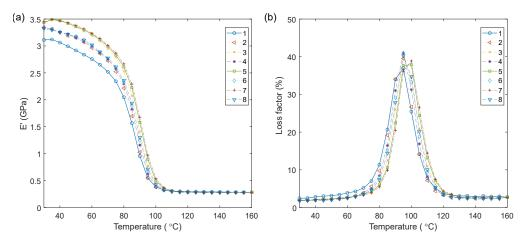
FIGURE II.13 – (a) Storage modulus and (b) loss factor of FGUD (post-curing at 130 °C and 1h) in transverse direction for each temperature cycles at 1 Hz
