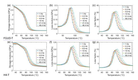
FIGURE II.22 – (a) Storage modulus, (b) loss modulus, (c) loss factor of FGUD-T at 1-50 Hz and 30 - 160 °C, (e) Storage modulus, (f) loss modulus, (g) loss factor of H4-T at 1-50 Hz and 30 - 160 °C
