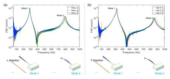
FIGURE III.18 – Modal response of H4 in (a) longitudinal direction, and (b) transverse direction
