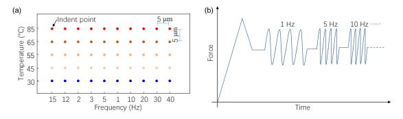
FIGURE IV.7 – Schematic diagram of nanoindentation for (a) GreenPoxy using the CAM protocol at 1 - 40 Hz and 30 - 85 °C (b) suggested protocol in the future plan
