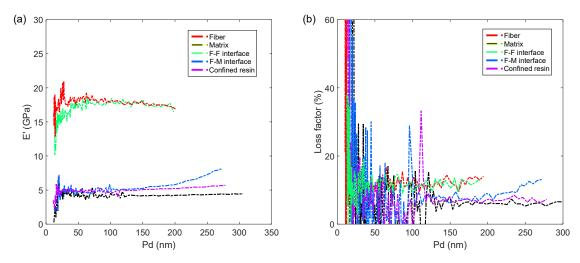
FIGURE IV.14 – Dependence on penetration depth of (a) the storage modulus and (b) loss factor obtained by typical CSM method at 5 Hz.
