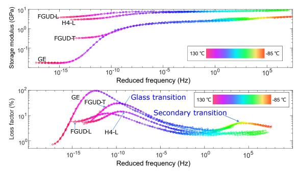
FIGURE II.25 – Master curves of storage modulus and loss factor for GE, FGUD and H4 with  $T_{ref}=25~{}^{\circ}{\rm C}$
