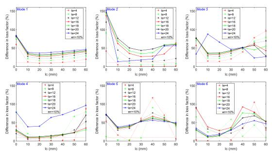
FIGURE III.8 – The influence of la and lc on mode 1-6 when lb=40 (Different curve refers to different value of la)
