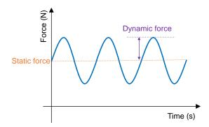
FIGURE II.5 – Excitation in DMA tests
