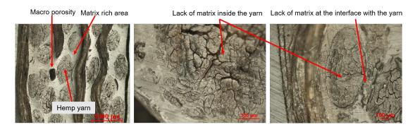
FIGURE II.19 – Mesostructure of H4/PA12
