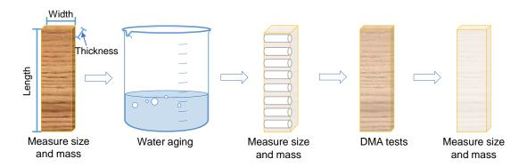
FIGURE II.10 – Water aging test process
