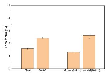
FIGURE III.13 – Comparison of the loss factor values determined for FUGD material in DMA and modal tests. (The results from DMA test is at 1 Hz and modal tests are obtained from the flexual modes in longitudinal direction (around 244 Hz) and transverse direction (204 Hz))
