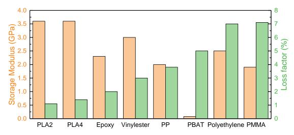
FIGURE I.5 – Loss factor and modulus of different polymers at 1 Hz and ambient temperature summarized from [Duc 14b, Margem 10, Ray 02, Shinoj 11, Madera-Santana 09, Martínez-Hernández 07, dos Santos Silva 19] (Polylactic acid 2, 4 (PLA 2, 4), and Polypropylene (PP), Polybutylene adipate-co-terephthalate (PBAT), Polymethyl methacrylate (PMMA))
