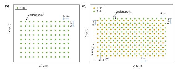
FIGURE IV.8 – Schematic diagram of nanoindentation for FGUD using (a) CSM at 5 Hz and (b) CAM method at 1 Hz and 5 Hz
