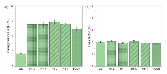
Figure II.18 – Comparison between balanced hemp fabric/GreenPoxy composites and FGCR in (a) storage modulus and (b) loss factor at 1 Hz and ambient temperature
