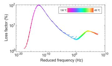
FIGURE II.24 – Master curve of loss factor for pure GE (reference temperature = 25 °C)
