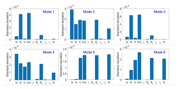
FIGURE III.11 – Standard deviation on loss factor obtained 5 % variation around the nominal value of the parameters in experimental setup (tick: thickness of the sample,  $\rho$ : density of the composites,  $E_t$  and  $E_l$ : Young's modulus in transverse and longitudinal direction,  $v_t$  and  $v_l$ : Possion's ratio in transverse and longitudinal direction, G: shear modulus)
