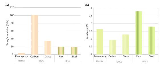
FIGURE I.3 – Mechanical properties of unidirectional (UD) fiber reinforced epoxy composites in the longitudinal direction (measured by DMA tests at 1 Hz and ambient temperature), summarized from refs. [Duc 14b, Mylsamy 11, Towo 08]
