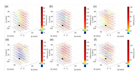
FIGURE III.10 – Difference of loss factor under various values of la, lb and lc in modes 1-6 ((a)-(g)) (the blue points refer to difference (err) is less than 10 %,  $\blacksquare$  refers to the final selected value)
