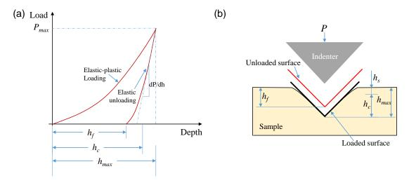
FIGURE IV.1 – (a) Typical loading-unloading curves ( $P_{max}$  is the maximum load during nanoindentation,  $h_f$  is the depth of the residual indentation,  $h_{max}$  is the depth from the original sample surface at load  $P_{max}$ ) (b) Profile change after indentation ( $h_s$  is the distance from the edge of the contact to the surface,  $h_s + h_c = h_{max}$ ,  $h_c$  is the contact depth measured from maximum depth  $h_{max}$ )
