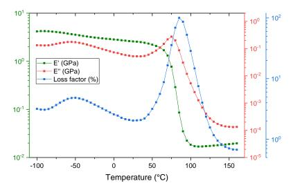
Figure II.15 – Dynamic mechanical properties of GreenPoxy from -100 to  $160~^{\circ}\mathrm{C}$  at 5 Hz
