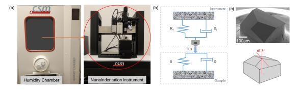
Figure IV.4 – (a) Anton Paar Nanoindentation Instrument (b) Dynamic mechanical model of viscoelastic material in the test system (c) Shape of Berkovich indenter [Fischer-Cripps 11]
