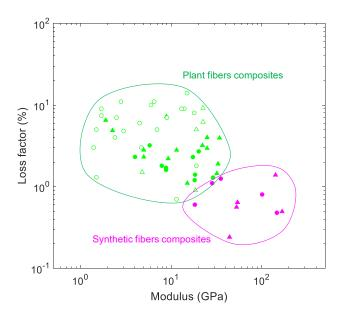
Figure I.10 – Ashby diagrams of PFCs and SFCs: loss factor v.s. modulus (triangles are measured by modal tests at first mode and ambient temperature, circles are measured by DMA tests at 1 Hz and ambient temperature, empty symbols and full symbols mean horizontal axis are using storage modulus and Young's modulus, respectively. (summarized from refs.
