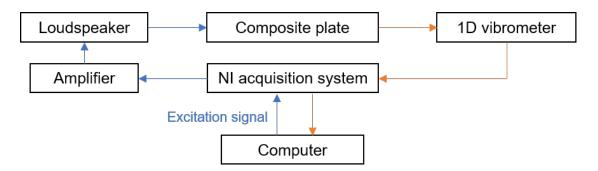
FIGURE III.4 – Schematic diagram of the experimental system
