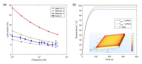
FIGURE IV.12 – (a) Comparison of loss factor in DMA and nanoindentation (NI) tests at the temperature near  $T_g$  zone (b) temperature changes based on numerical model
