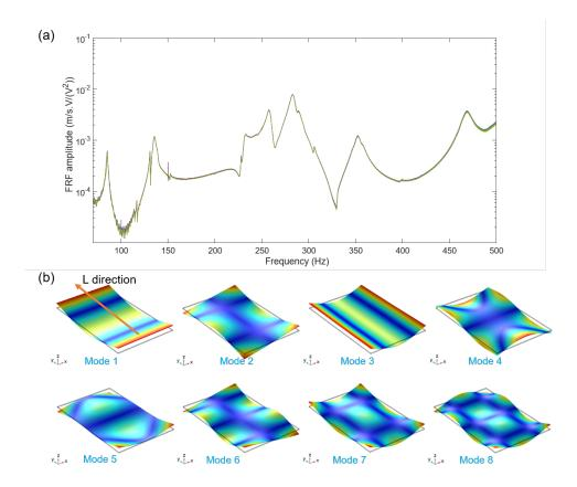
FIGURE III.15 – (a) FRF from numerical model and experiment, and (b) modal shape in numerical model for H4 in free-free condition
