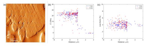
FIGURE IV.20 – (a) Micro-structure on the cross section after nanoindentation tests, (b) storage modulus and (c) loss factor at 1 Hz and 5 Hz versus distance from each fiber edge
