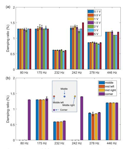
FIGURE A.1 – Influence of (a) amplitude of excitation and (b) position of measurement on the damping ratio identification under free-free boundary condition
