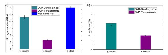
FIGURE II.11 – (a) Storage modulus and (b) loss factor of FGUD-L obtained from DMA test in bending and tension mode at 1 Hz (E-Static refers to monotonic test in tension)
