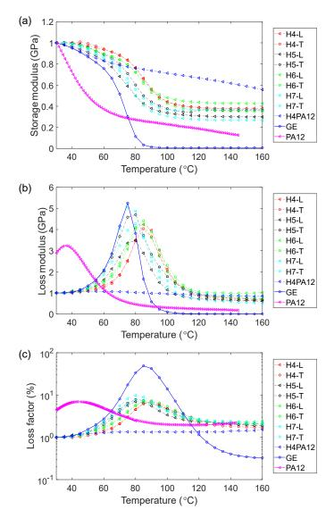
FIGURE II.21 – (a) Normalized storage modulus, (b) loss modulus, (c) loss factor of HFRC at 1 Hz and 30 - 160 °C (PA12 is collected from Ref. [Liao 18])
