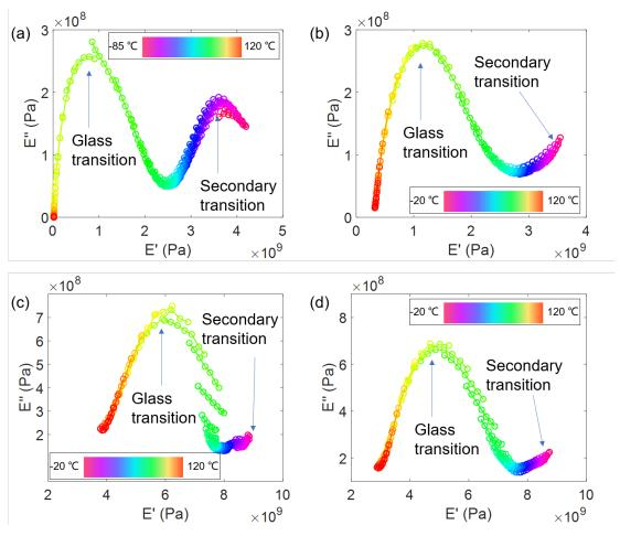
Figure II.26 – Cole-cole curve of (a) GE, (b) FGUD-T, (c) FGUD-L and (d)  $\rm H4\text{-}L$
