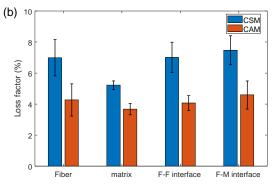
FIGURE IV.23 – Comparison of (a) storage modulus and (b) loss factor at 5 Hz obtained from CSM and CAM method on the same sample
