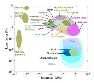
FIGURE I.1 – Ashby diagram: loss factor v.s. modulus at ambient temperature (summarized from
