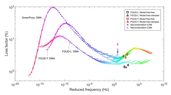
FIGURE IV.25 – Comparison of loss factor in GreenPoxy identified from DMA tests, FGUD identified from DMA and modal tests and fiber zone identified from nanoindentation tests based on CAM and CSM method using the average value
