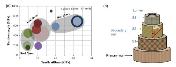
FIGURE 5 – (a) Absolute tensile properties of different series of fiber [Shah 14] (b) The schematic representation of the flax and hemp fiber structure
