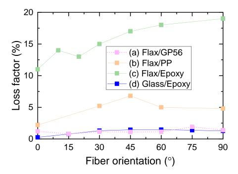
FIGURE I.4 – Variation of loss factor as function of fiber orientation in UD composites in longitudinal direction using modal tests (a) Flax/GP56, (b)
