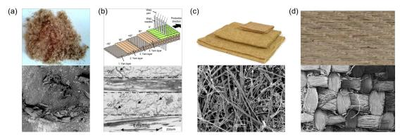
Figure 6 – Different reinforcements and micro-structures of (a) short fiber [Datta 17] (b) non-crimp [Schrank 17, Liang 14](c) non-woven [Reinders, Martin 16] and (d) woven fabric [Song 12, Corbin 20b]
