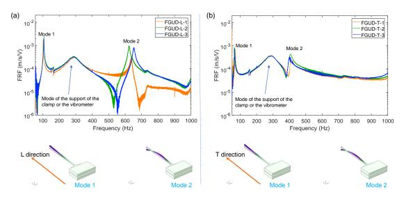
FIGURE III.16 – Modal response of FGUD in (a) longitudinal direction, and (b) transverse direction
