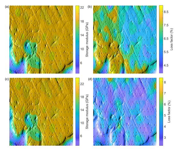
FIGURE IV.22 – Map on the cross section based on the results from storage modulus and loss factor at 5 Hz using (a) - (b) CSM and (c) - (d) CAM method on the same sample
