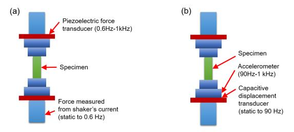
FIGURE II.4 – (a) Force measurement and (b) displacement measurement technologies in the used device
