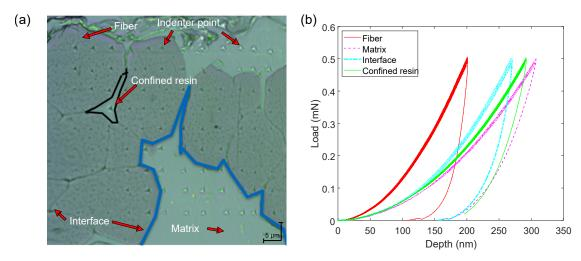
FIGURE IV.13 – Static mechanical properties of FGUD (a) microstructure on the surface (b) experimental loading-unloading curves for different zones (confined resin is in the closed boundary with black line)
