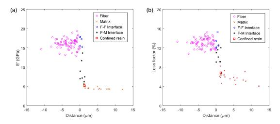
FIGURE IV.17 – (a) Storage modulus and (b) loss factor at 5 Hz versus distance from each fiber edge
