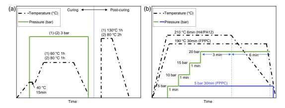
FIGURE II.9 – Temperature and pressure during fabrication of (a) (1) pure GreenPoxy and plant fiber/GreenPoxy composites (2) Pure petro-based epoxy and plant fiber/petro-based epoxy composites, (b) Hemp/PA12 composites
