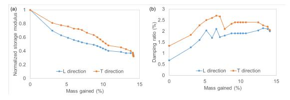
FIGURE III.23 – Results of water aging tests for (a) normalized storage modulus and (b) loss factor as a function of gained mass in L and T direction
