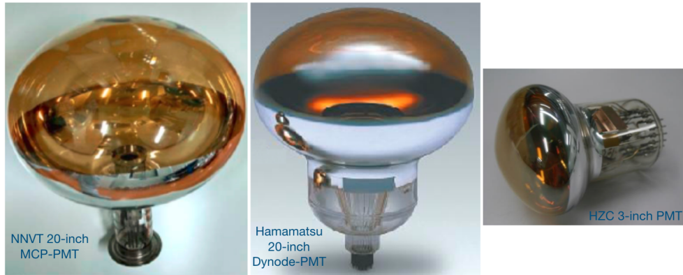
Figure 3.3 – Photos of the JUNO LPMTs and SPMT. Left: NNVT 20-inch MCP-PMT. Middle: Hamamatsu 20-inch Dynode-PMT. Right: HZC 3-inch PMT.
