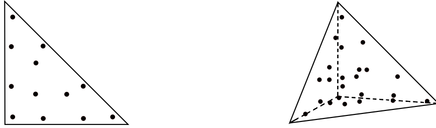
(a) Quadrature points on 2D reference elements. (b) Quadrature points on 3D reference elements.
