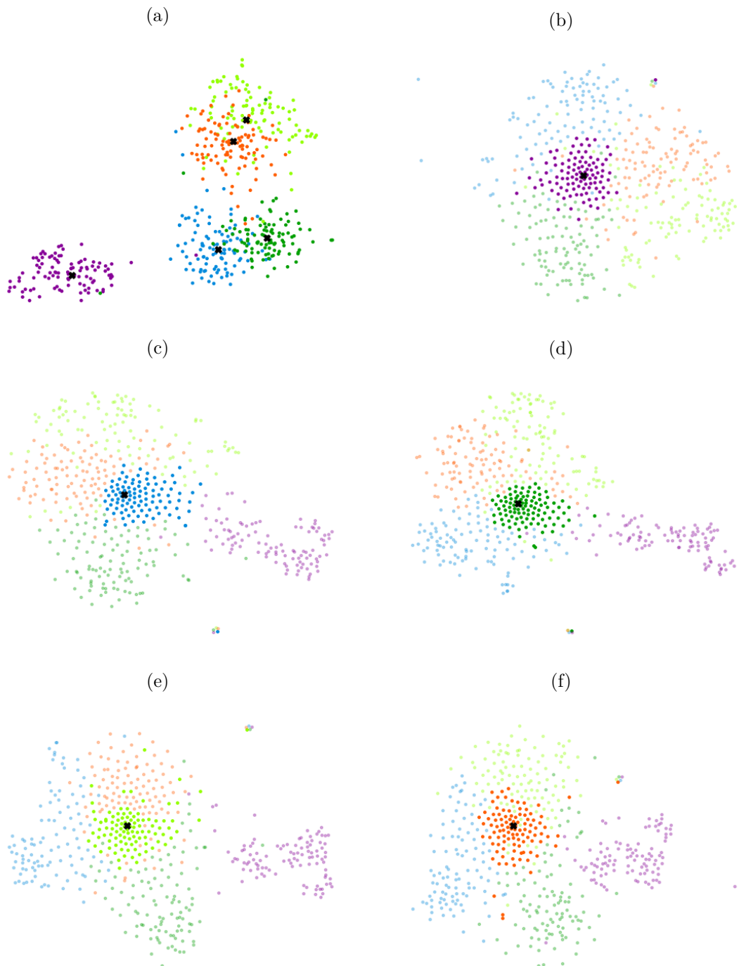
Figure 4.4: t-SNE projections of feature spaces for five classes from CIFAR-100 test set (colors are given by the ground truth). (a): feature space before applying INNs (black crosses are the clusters centers). (b),(c),(d),(e),(f): each feature space after the INN of each class. The samples of a class represented by a network are clustered around the zero vector (black cross) whilst the samples from other classes appear further away from the cluster.
