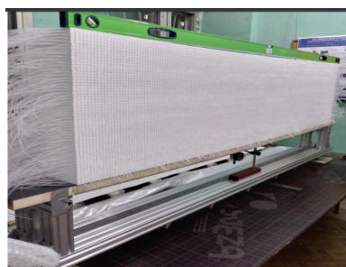
Figure 8.6: The tall prototype of the SuperFGD detector made with 15 \times 56 \times 192 cubes.
