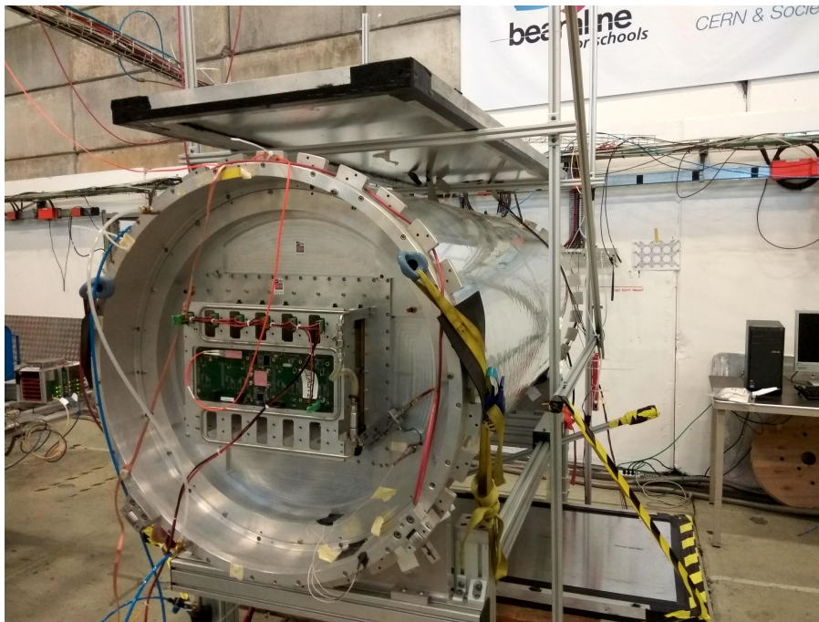
Figure 7.10: The photo of the TPC prototype installed at the CERN beamline. The Micromegas are installed in the closes end cap of the cylinder field cage. The scintillator planes for the cosmic trigger are put above and below the TPC.
