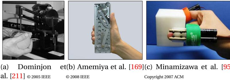
Figure 2.40: Enhanced weight of tangibles: (a) Influence of Control/Display Ratio [211], (b) Asymmetric Oscillation Distorts the Perceived Heaviness [169], (c) Gravity Grabber [95].
