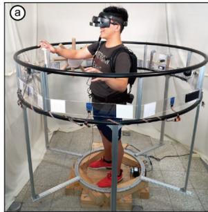
Figure 2.5: Encounter-Type using Encasing Structure: Haptic-Go-Round [59] Copyright 2020 ACM.
