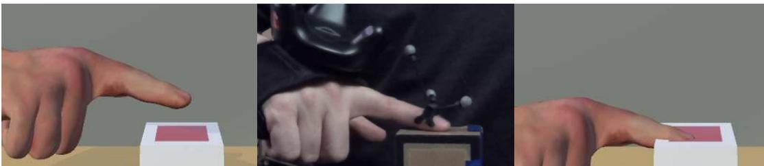
Figure 6.1: Exaggerated examples of discrepancies upon tangible contact: as the user is touching the tangible object (middle), there can be a virtual gap (left) or virtual interpenetration (right) between the virtual finger and the virtual object's surface.
