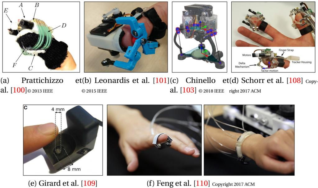
Figure 2.16: Compact wearable devices. (a) Towards Wearability in Fingertip Haptics [100], (b) 3-RSR [101], (c) 3-RRS [103], (d) Fingertip Tactile Devices [108], (e) HapTip [109], (f) Submerged Haptics [110].
