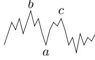
Figure 1.2: Potential with a trap between b and c with a minimum in a
