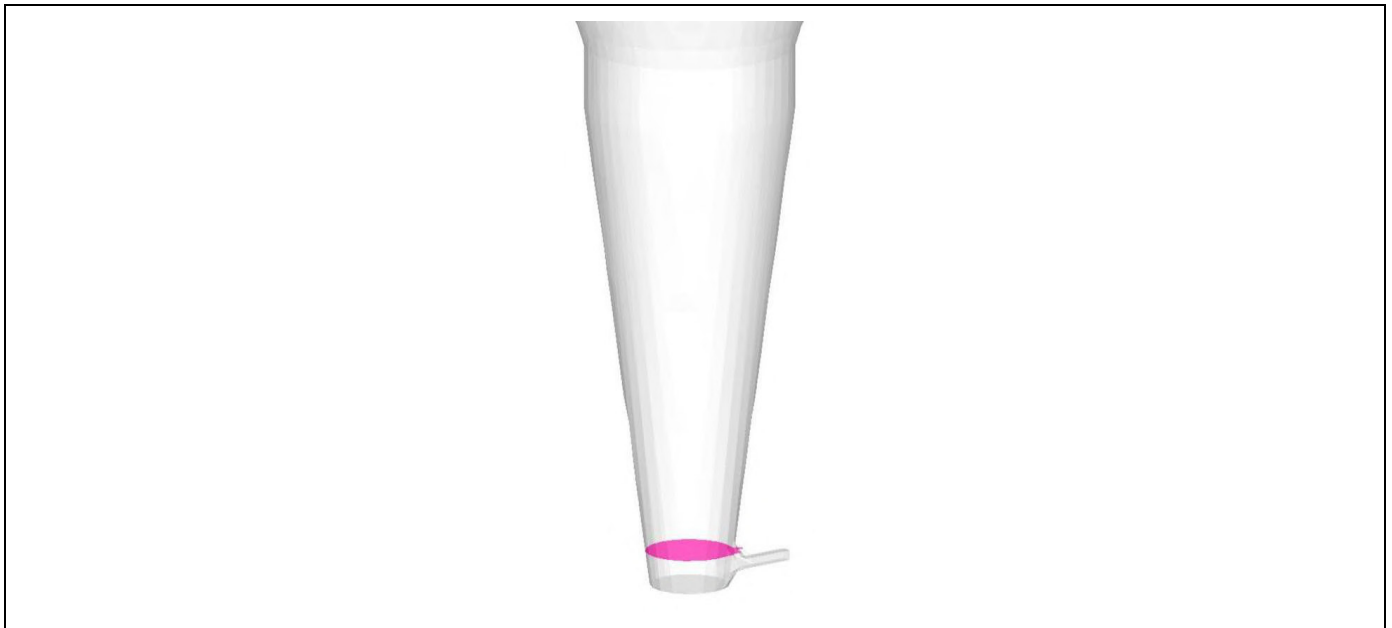
Figure II-10 : Virtual plane above the air injection to evaluate the solid circulation
