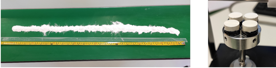
Figure 8.5 – Ground powder spread out for the sampling procedure (left) and pellets obtained after compacting (right).
