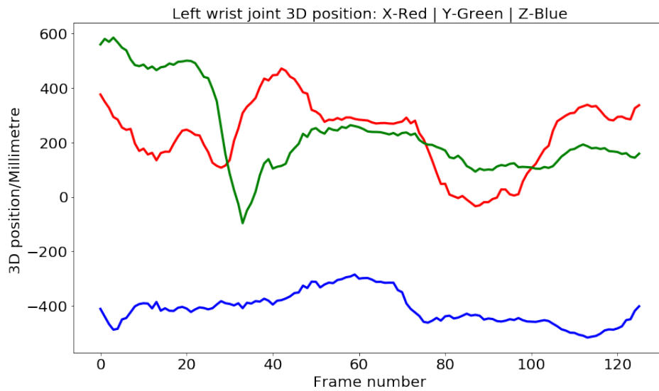
Figure 2.14: 3D position plot of left wrist joint.
