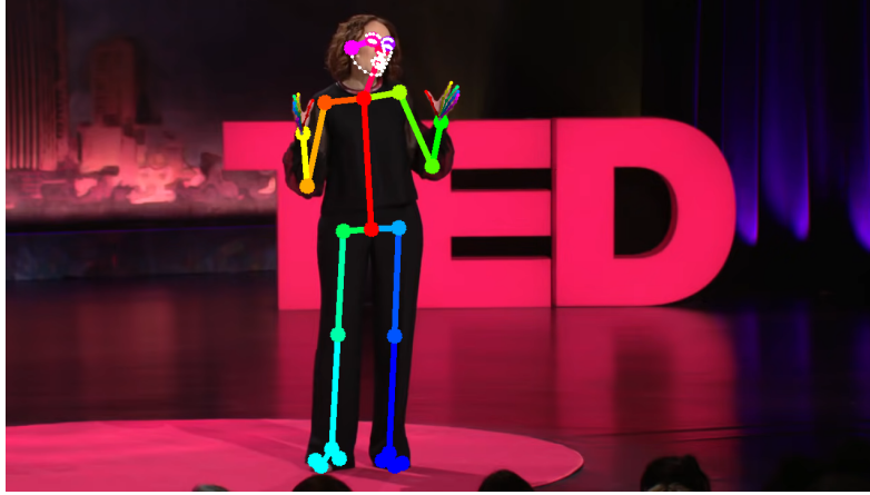
Figure 2.10: OpenPose for whole-body estimation.
