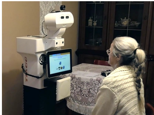
Figure 1.2: Human-robot interaction with the elderly in the project ENRICHME. The robot TIAGo monitors the health situation of the elderly and interact with the old people [64].
