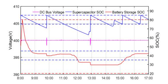
Figure 85. The ideal results of DC bus voltage and BS SOC curves at full microgrid mode on May 8<sup>th</sup> 2018.
