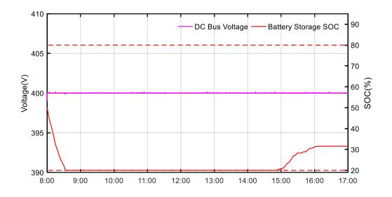
Figure 37. DC bus voltage and BS SOC curves when  $k_D = 0$  at grid-connected mode on May 8<sup>th</sup> 2018.
