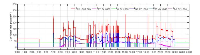
Figure 129. The converter loss power curves of case 3 at full microgrid mode on June 20<sup>th,</sup> 2018. In Figure 129, the power loss curves of the converter of case 3 are shown. The power loss varies
