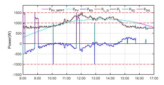
Figure 64. The ideal results of power curves at off-grid mode on May 8<sup>th</sup> 2018.
