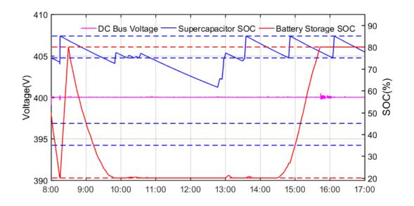
Figure 75. DC bus voltage and BS SOC curves when  $k_D = 1$  and  $k_{DG} = 0$  at full microgrid mode on May 8<sup>th</sup> 2018.
