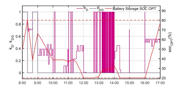
Figure 69. The day-ahead economics optimization results ( $k_D$ ,  $k_{DG}$ ) and BS SOC curves at full microgrid mode on May 8<sup>th</sup> 2018.
