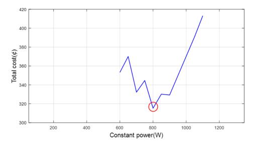
Figure 43. The total cost with constant DG power at off-grid mode on May 8<sup>th</sup> 2018.
