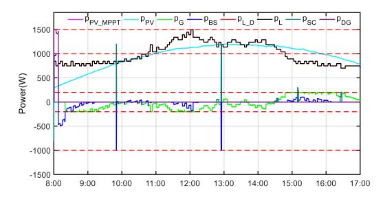
Figure 88. The actual results of power curves at full microgrid mode on May 8<sup>th</sup> 2018.
