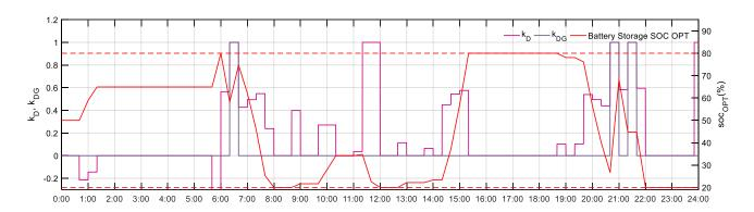
Figure 117. The day-ahead economics optimization results  $k_D$ ,  $k_{DG}$  and BS SOC curves at full microgrid mode on June 20<sup>th,</sup> 2018 without converter loss.
