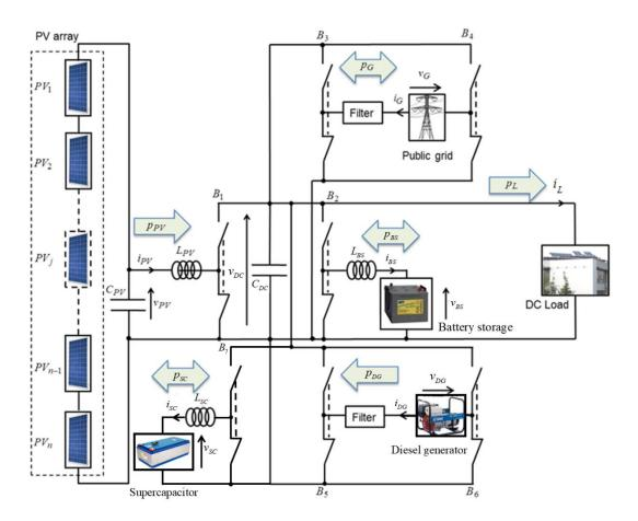
Figure 3. DC microgrid electrical scheme [53].
