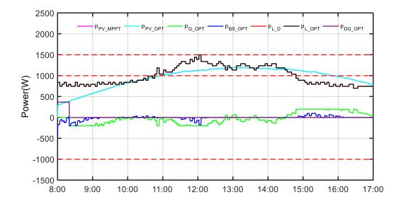
Figure 74. The ideal economics optimization results of power curves at full microgrid mode on May  $8^{th}$  2018.
