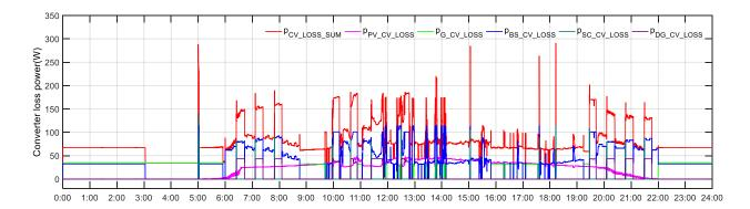
Figure 126. The converter loss power curves of case 2 at full microgrid mode on June 20<sup>th</sup>, 2018.
