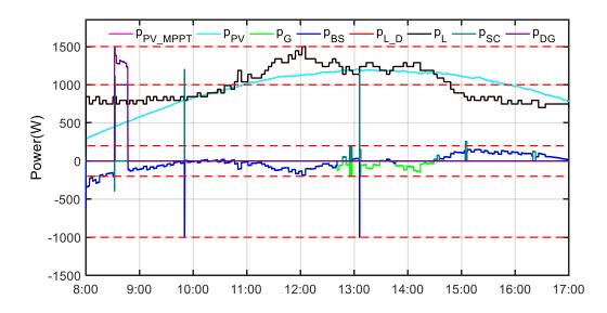
Figure 78. Power curves when  $k_D = 0.5$  and  $k_{DG} = 0$  at full microgrid mode on May 8<sup>th</sup> 2018. The results when  $k_D$  equal to 0 and  $k_{DG}$  equal to 0 are shown in Figure 79 and Figure 80. In Figure 79 and Figure 80, the DG is turned on at 8:32; the SC is recharging at 9:55, 12:45, 12:55, 14:30, 15:05, and 16:20, there is no load shedding and PV shedding.
