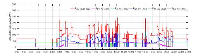
Figure 135. The converter loss power curves of case 5 at full microgrid mode on June 20<sup>th,</sup> 2018.
