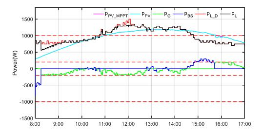
Figure 34. Power curves when  $k_D = 1$  at grid-connected mode on May 8<sup>th</sup> 2018.
