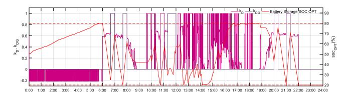
Figure 97. The ideal economics optimization results ( $k_D$ ,  $k_{DG}$ ) and BS SOC curves at full microgrid mode on June 20<sup>th</sup> 2018.
