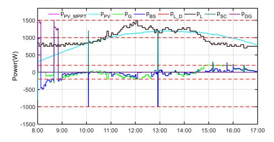
Figure 82. The actual results of power curves at full microgrid mode on May 8<sup>th</sup> 2018.
