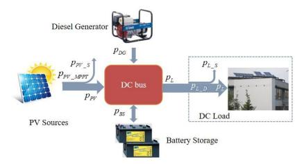
Figure 7. Off-grid microgrid power flow.
