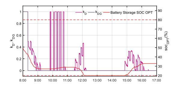
Figure 73. The ideal economics optimization results ( $k_D$ ,  $k_{DG}$ ) and BS SOC curves at full microgrid mode on May 8<sup>th</sup> 2018.
