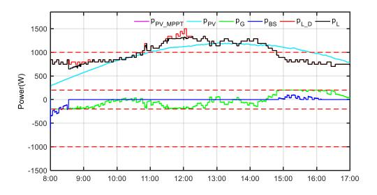
Figure 38. Power curves when  $k_D = 0$  at grid-connected mode on May 8<sup>th</sup> 2018.
