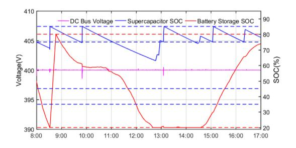
Figure 77. DC bus voltage and BS SOC curves when  $k_D = 0.5$  and  $k_{DG} = 0$  at full microgrid mode on May 8<sup>th</sup> 2018.
