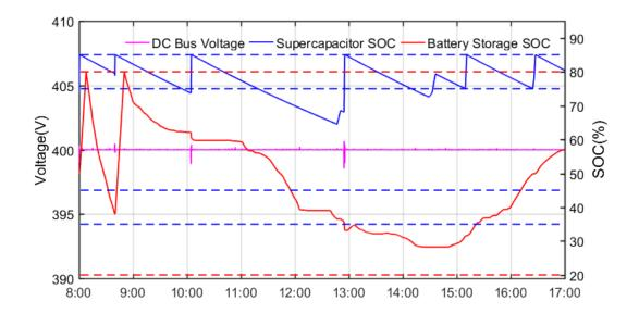
Figure 83. The actual results of DC bus voltage and BS SOC curves at full microgrid mode on May 8<sup>th</sup> 2018.
