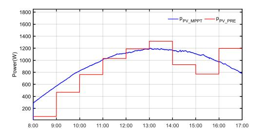
Figure 25. PV MPPT power and PV prediction power curves for May 8<sup>th</sup> 2018.
