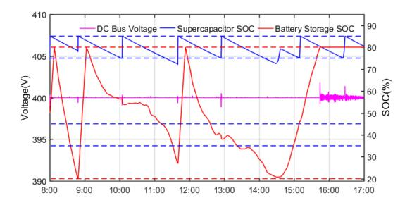
Figure 65. The ideal results of DC bus voltage and BS SOC curves at off-grid mode on May 8<sup>th</sup> 2018.
