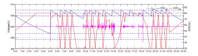
Figure 124. DC bus voltage and BS SOC curves of case 2 at full microgrid mode on June 20<sup>th,</sup> 2018.
