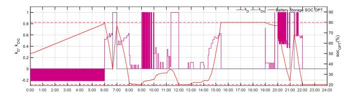
Figure 91. The day-ahead economics optimization results ( $k_D$ ,  $k_{DG}$ ) and BS SOC curves at full microgrid mode on June 20<sup>th</sup> 2018.
