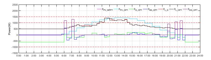
Figure 120. The day-ahead economics optimization results of power curves at full microgrid mode on June 20<sup>th.</sup> 2018 with converter loss.
