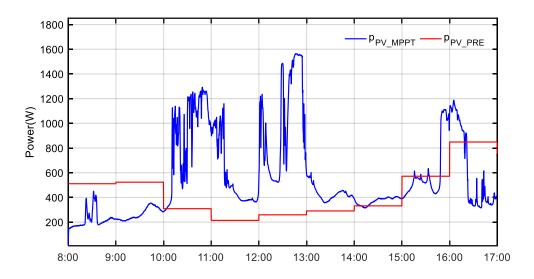
Figure 27. PV MPPT power and PV prediction power curves for July 16<sup>th</sup> 2018. The load demand power and load power prediction curves are given in Figure 28.
