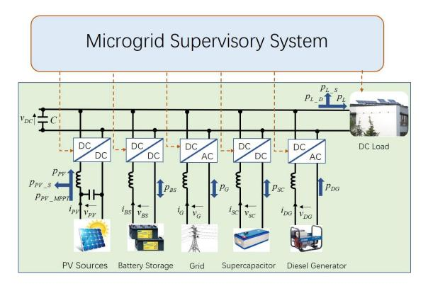
Figure 4. Microgrid multi-layer supervisory concept.
