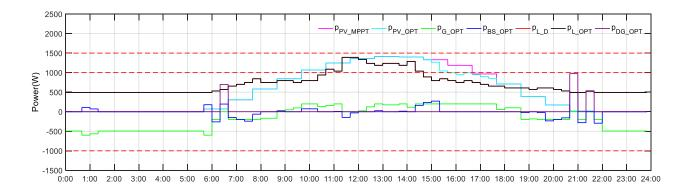
Figure 118. The day-ahead economics optimization results of power curves at full microgrid mode on June 20<sup>th,</sup> 2018 without converter loss.
