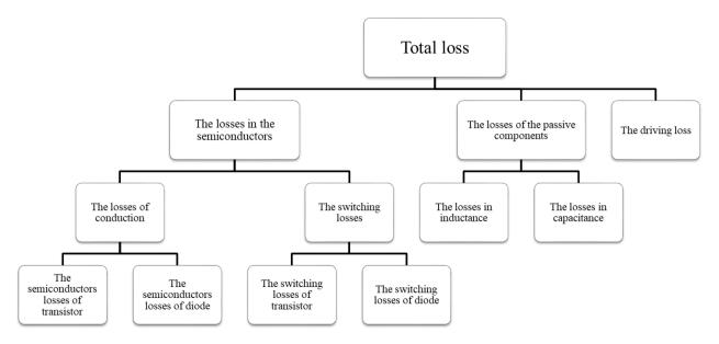
Figure 111. Power loss classification in the converter.
