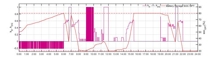
Figure 93. The day-ahead economics optimization results ( $k_D$ ,  $k_{DG}$ ) and BS SOC curves at full microgrid mode on June 20<sup>th</sup> 2018.
