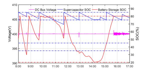
Figure 61. The actual results of DC bus voltage and BS SOC curves at off-grid mode on May 8<sup>th</sup> 2018.
