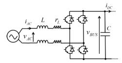
Figure 110. The single-phase full-bridge DC/AC converter.
