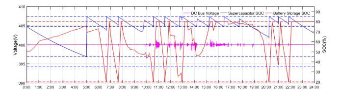
Figure 103. The actual results of DC bus voltage and BS SOC curves at full microgrid mode on June  $20^{\text{th}} 2018$ .
