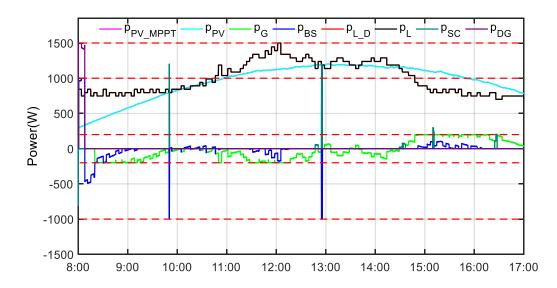
Figure 86. The ideal results of power curves at full microgrid mode on May 8<sup>th</sup> 2018.
