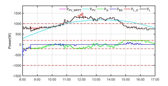
Figure 42. The ideal results of power curves at grid-connected mode on May 8<sup>th</sup> 2018.
