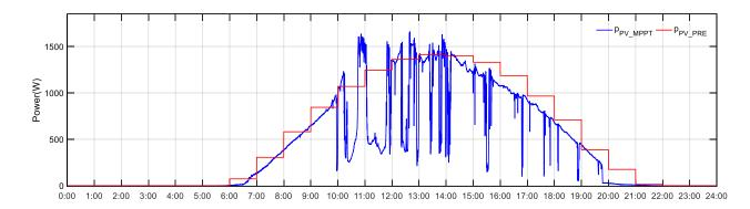
Figure 89. PV MPPT power and PV prediction power curves for June 20<sup>th</sup> 2018. The load power and load power prediction curves are given in Figure 90 are used.
