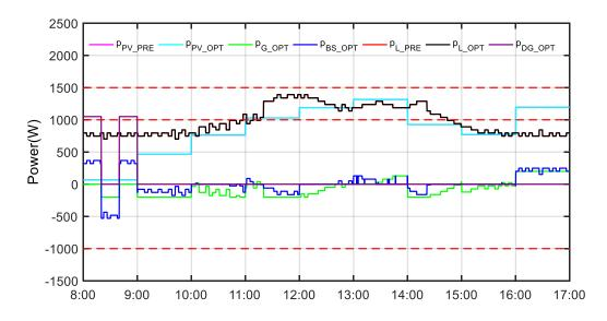
Figure 68. The day-ahead economics optimization results of power curves at full microgrid mode on May 8<sup>th</sup> 2018.
