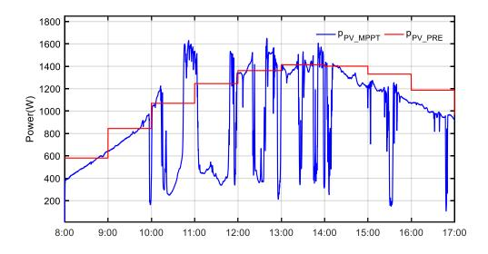
Figure 26. PV MPPT power and PV prediction power curves for June 20<sup>th</sup> 2018.
