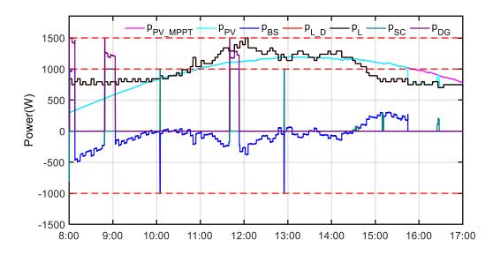
Figure 66. The ideal results of power curves at off-grid mode on May 8<sup>th</sup> 2018.
