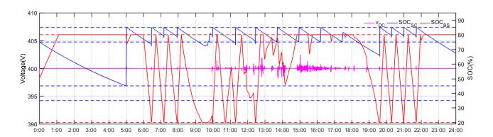
Figure 122. DC bus voltage and BS SOC curves of case 1 at full microgrid mode on June 20<sup>th,</sup> 2018.
