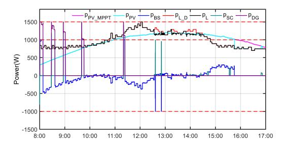
Figure 60. The actual results of power curves at off-grid mode on May 8<sup>th</sup> 2018.
