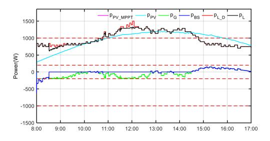
Figure 36. Power curves when  $k_D = 0.5$  at grid-connected mode on May 8<sup>th</sup> 2018.
