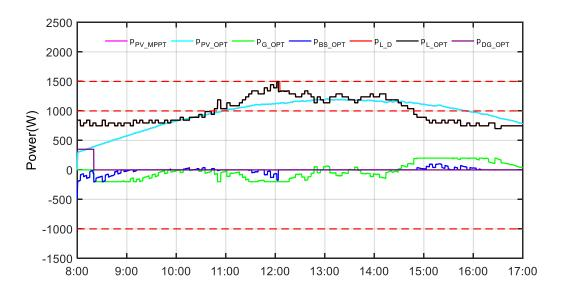
Figure 72. The ideal economics optimization results of power curves at full microgrid mode on May 8<sup>th</sup> 2018.
