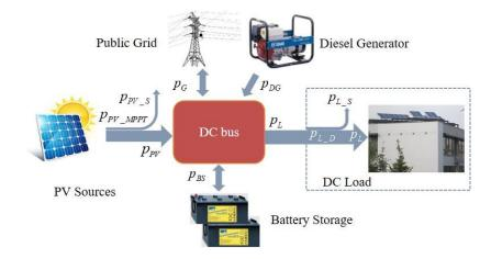
Figure 8. Full microgrid power flow.
