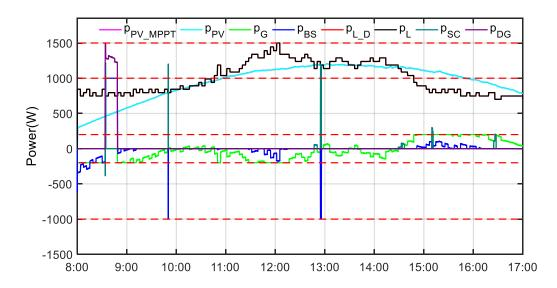
Figure 80. Power curves when  $k_D = 0$  and  $k_{DG} = 0$  at full microgrid mode on May 8<sup>th</sup> 2018.
