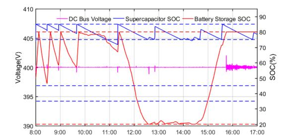
Figure 59. The actual results of DC bus voltage and BS SOC curves at off-grid mode on May 8<sup>th</sup> 2018.
