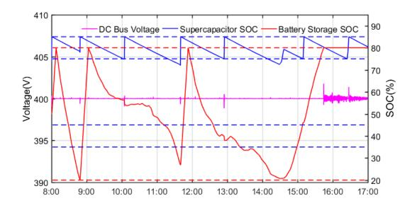
Figure 63. The ideal results of DC bus voltage and BS SOC curves at off-grid mode on May 8<sup>th</sup> 2018.
