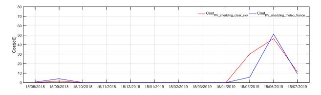
Figure 137. The PV shedding cost comparison between the clear sky model and the Météo France model.
