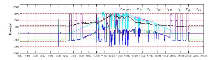
Figure 123. Power curves of case 1 at full microgrid mode on June 20<sup>th,</sup> 2018. The simulation results of case 2 are shown in Figure 124, Figure 125, and Figure 126.
