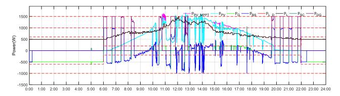
Figure 100. Power curves when  $k_D = 1$  and  $k_{DG} = 0$  at full microgrid mode on June 20<sup>th</sup> 2018.
