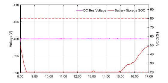
Figure 39. The actual results of DC bus voltage and BS SOC curves at grid-connected mode on May 8<sup>th</sup> 2018.
