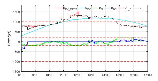
Figure 40. The actual results of power curves at grid-connected mode on May 8<sup>th</sup> 2018.
