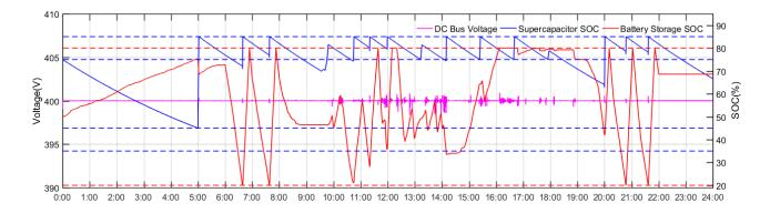
Figure 107. The actual results of DC bus voltage and BS SOC curves at full microgrid mode on June  $20^{\text{th}} 2018$ .
