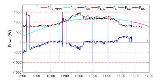
Figure 58. Power curves when  $k_{DG} = 0$  in off-grid mode on May 8<sup>th</sup> 2018.
