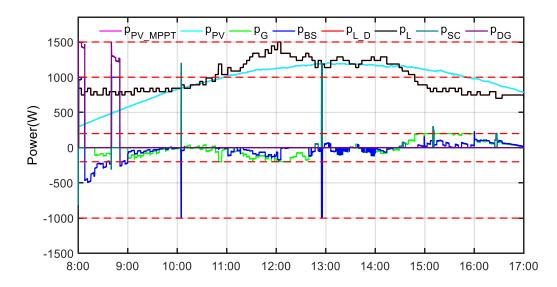
Figure 84. The actual results of power curves at full microgrid mode on May 8<sup>th</sup> 2018.
