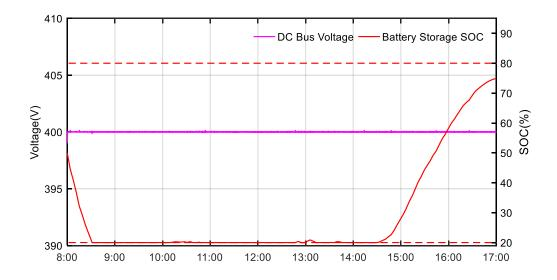
Figure 35. DC bus voltage and BS SOC curves when  $k_D = 0.5$  at grid-connected mode on May 8<sup>th</sup> 2018.
