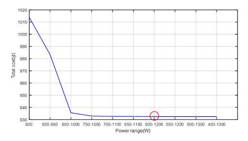
Figure 48. The total cost with variable DG power at off-grid mode on July 16<sup>th</sup> 2018.
