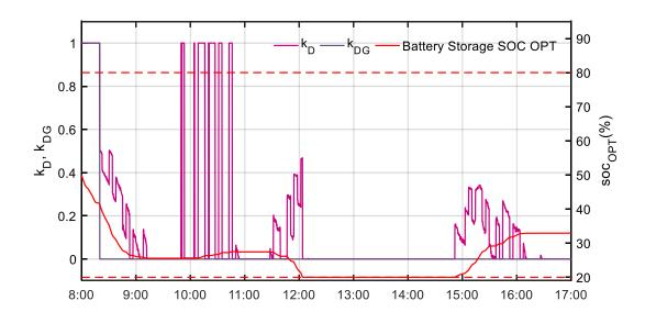
Figure 71. The ideal economics optimization results ( $k_D$ ,  $k_{DG}$ ) and BS SOC curves at full microgrid mode on May 8<sup>th</sup> 2018.
