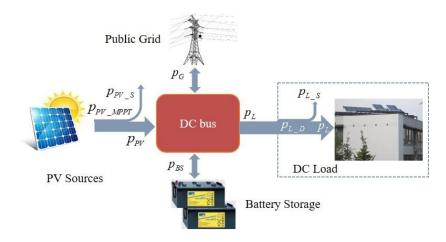
Figure 6. Grid-connected microgrid power flow.
