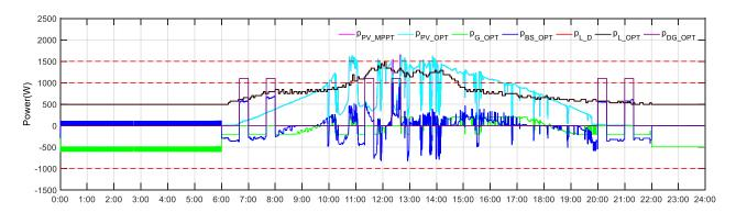
Figure 96. The ideal economics optimization results of power curves at full microgrid mode on June  $20^{\text{th}} 2018.$
