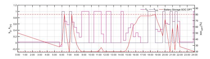
Figure 119. The day-ahead economics optimization results  $k_D$ ,  $k_{DG}$  and BS SOC curves at full microgrid mode on June 20<sup>th,</sup> 2018 with converter loss.
