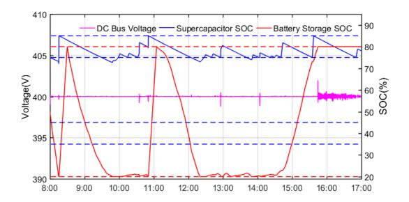
Figure 57. DC bus voltage and BS SOC curves when  $k_{DG} = 0$  at off-grid mode on May 8<sup>th</sup> 2018.
