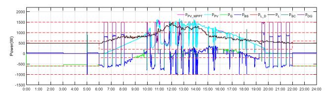
Figure 125. Power curves of case 2 at full microgrid mode on June 20<sup>th</sup>, 2018.
