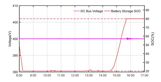
Figure 33. DC bus voltage and BS SOC curves when  $k_D = 1$  at grid-connected mode on May 8<sup>th</sup> 2018.
