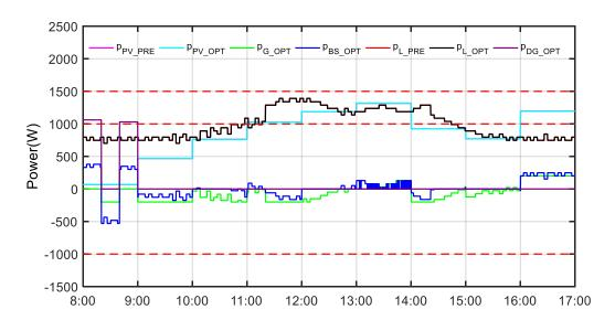
Figure 70. The day-ahead economics optimization results of power curves at full microgrid mode on May 8<sup>th</sup> 2018.
