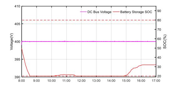
Figure 41. The ideal results of DC bus voltage and BS SOC curves at grid-connected mode on May 8<sup>th</sup> 2018.
