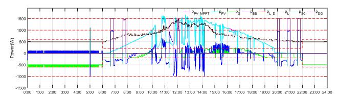
Figure 108. The actual results of power curves at full microgrid mode on June 20<sup>th</sup> 2018.
