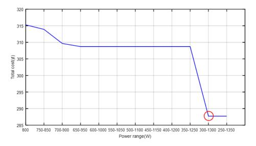
Figure 44. The total cost with variable DG power at off-grid mode on May 8<sup>th</sup> 2018.
