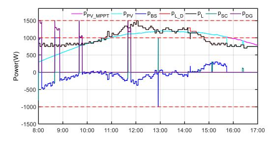
Figure 62. The actual results of power curves at off-grid mode on May 8<sup>th</sup> 2018.
