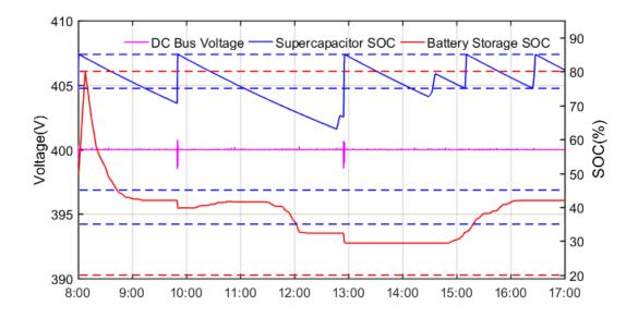
Figure 87. The actual results of DC bus voltage and BS SOC curves at full microgrid mode on May 8<sup>th</sup> 2018.
