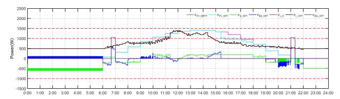
Figure 92. The day-ahead economics optimization results of power curves at full microgrid mode on June  $20^{th} 2018$ .
