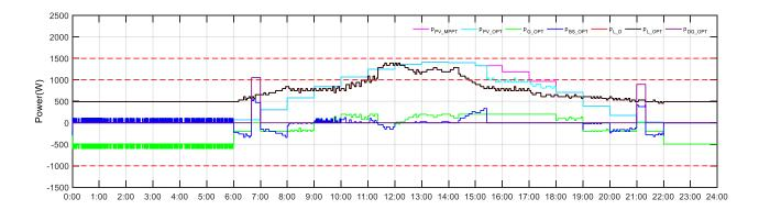
Figure 94. The day-ahead economics optimization results of power curves at full microgrid mode on June  $20^{\text{th}} 2018$ .
