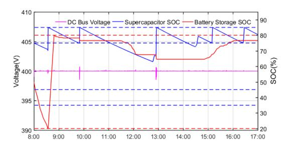
Figure 79. DC bus voltage and BS SOC curves when  $k_D = 0$  and  $k_{DG} = 0$  at full microgrid mode on May 8<sup>th</sup> 2018.
