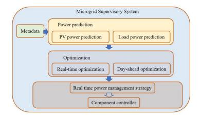
Figure 136. The supervisory system structure in a full DC microgrid with the power prediction model.
