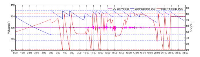
Figure 105. The ideal results of DC bus voltage and BS SOC curves at full microgrid mode on June  $20^{\text{th}} 2018$ .
