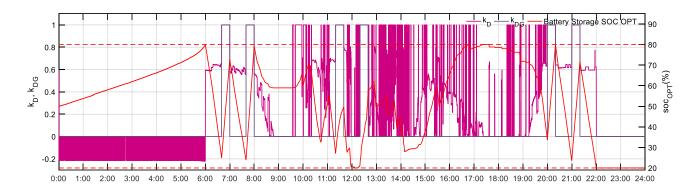
Figure 95. The ideal economics optimization results ( $k_D$ ,  $k_{DG}$ ) and BS SOC curves at full microgrid mode on June 20<sup>th</sup> 2018.
