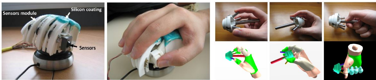
FIGURE A.13 – Left : The HandNavigator. Right : Several examples of finger configuration to grasp the same object, in the real world and in virtual reality. Green parts correspond to parts colliding with the virtual object.
