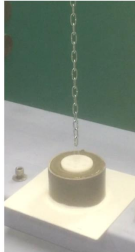
Figure 35. Photography of one disc situated on mortar surface and pulled-off with the traction machine.
