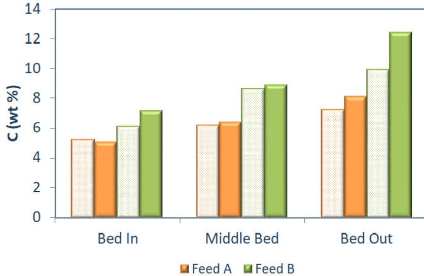
Figure 54. Carbon content of the spent catalysts. Samples taken at different reactor locations. Full bars=30 days tests, open bars=6 days tests.
