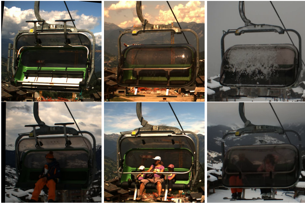
Figure 6.6 – Examples of images of chairlift C_0 . In the images of the first row, the chairlift carrier is empty, while in the second row, it is occupied. The safety bar is in different positions and so on the protection class (open or closed).
