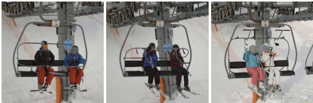
Figure 1 – Chairlifts leaving the boarding station in three situations 1 , from left to right: (i) passengers have fully closed the safety bar ( safe ), (ii) passengers are closing the bar ( unsafe ), (iii) passengers did not close the bar ( unsafe ).
