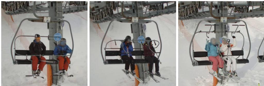
Figure 1 – Chairlifts leaving the boarding station in three situations<sup>1</sup>, from left to right: (i) passengers have fully closed the safety bar (*safe*), (ii) passengers are closing the bar (*unsafe*), (iii) passengers did not close the bar (*unsafe*).
