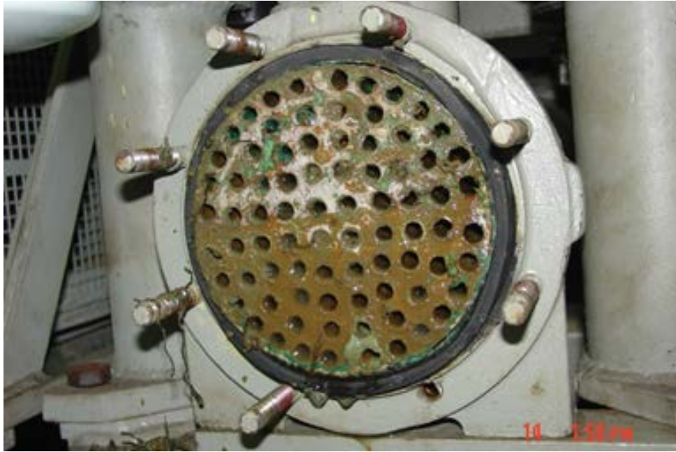
FIGURE 1.1 – Photo of fouled inner surfaces of tubular heat exchanger used in a ship (Navy Currents Winter 2015)
