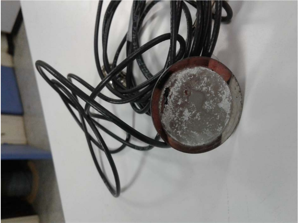
FIGURE 3.13 – Protein fouling layer formed on the substrate
