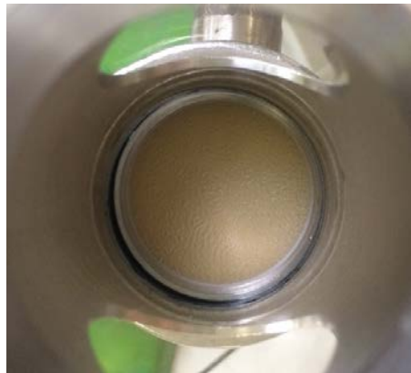
FIGURE 4.2 – Photo of biofilm formed on the substrate of reactor 1
