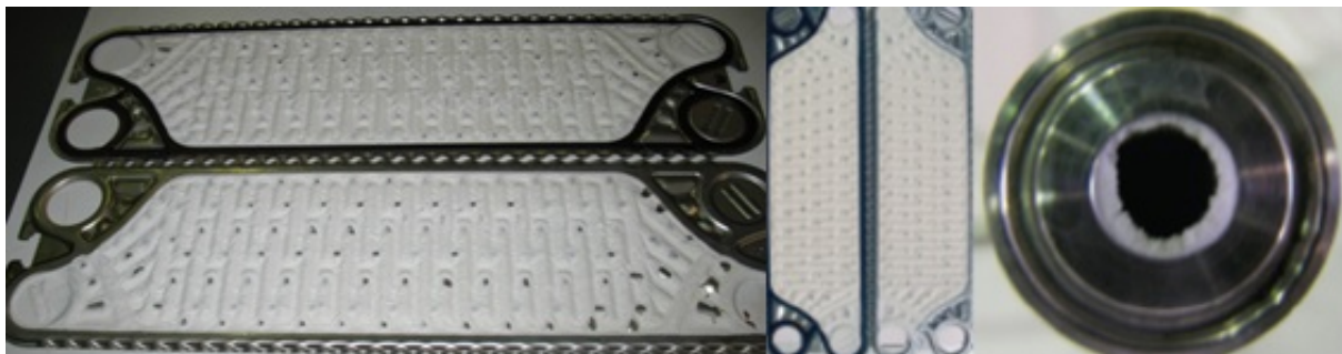
FIGURE 1.3 – Deposit on inner surfaces of heat treatment equipment ; heat exchanger in form of plate (left) ; heat exchanger in form of tube (right)
