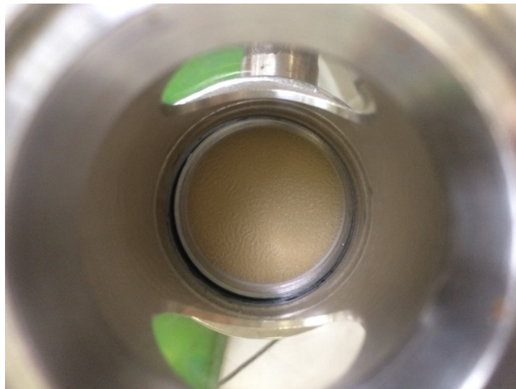
FIGURE 1.4 – Bacterial biofilm on a stainless steel substrate
