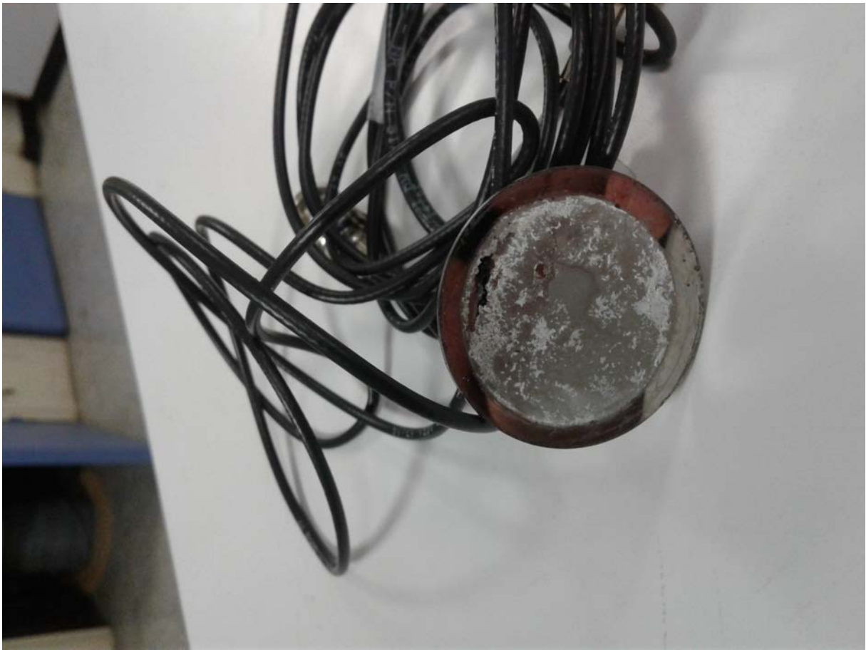
FIGURE 3.13 – Protein fouling layer formed on the substrate
