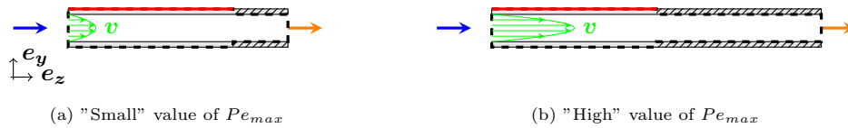
Figure 8: Test Pe_{max} in the exchanger configuration. In this illustration, a variation of the velocity is shown, but other parameters can influence this parameter, such as the conductivity of the fluid or the dimension of the duct. As Pe_{max} changes, the extended zone down the flow is also extended.
