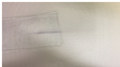
Figure 5.13: Photograph of the irradiated surface of [C_{20}mim]^+[NTf_2]^- Langmuir film deposited on a subphase containing 30 [AuCl_4]^-/IL for 8 hours.
