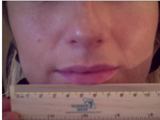
Figure 6.6: Lip dimension measures in world units. A straight horizontal line (in yellow) was positioned along an image of a physical ruler for a distance of 10 cm.
