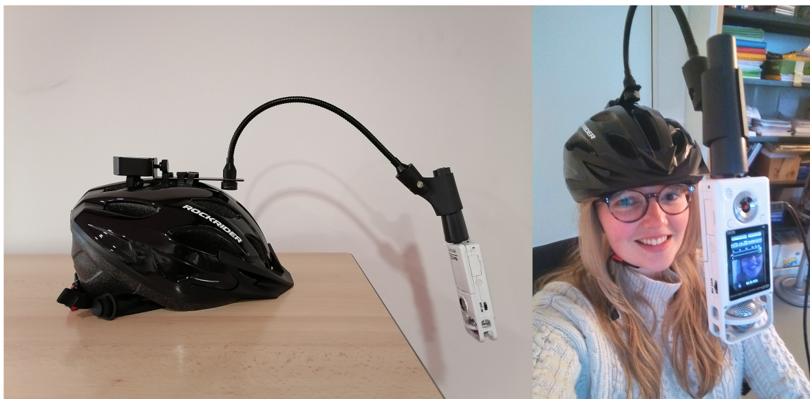
Figure 6.1: The author demonstrating video camera stabilisation using a bike helmet, a flexible arm and a handheld tripod.
