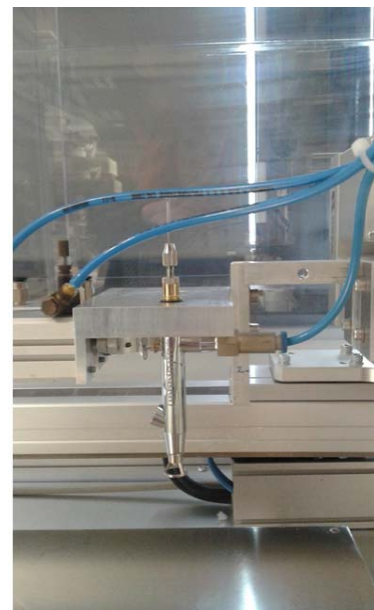
Figure A-1: Photo of the Airbrush with its main parts (left), placed inside the spray coating set-up (right).
