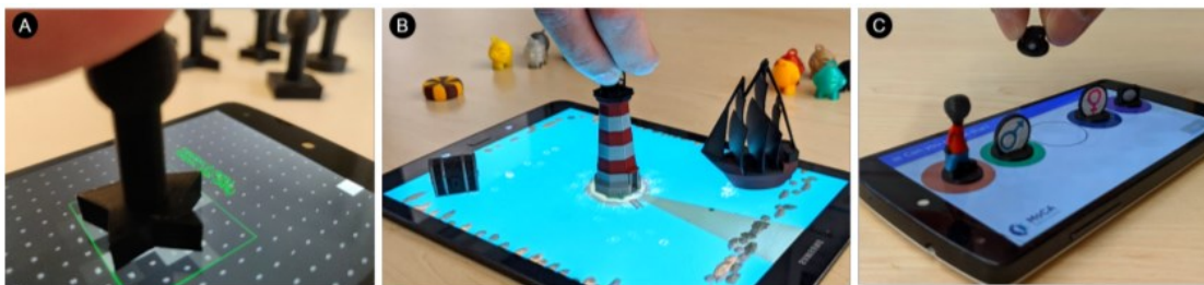
Figure 109. Itsy-Bits recognizes 3D-printed tangible objects via the capacitive touchscreen.
