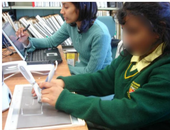
Figure 40. The system McSig [104]. The teacher on the left draws on a Tablet PC to create a shape and the student on the right can feel, explore and be moved around the shape.
