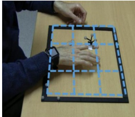
Figure 4. A blind user exploring an invisible digital map based on movement tracking [13].
