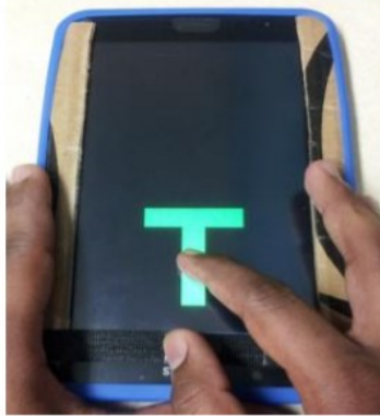
Figure 30. Exploring a T-like digital graphic with vibro-audio mode [37].
