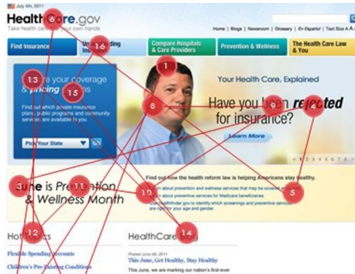
Figure 73. A series of consecutive eye fixations reveal the user's eye movements.
