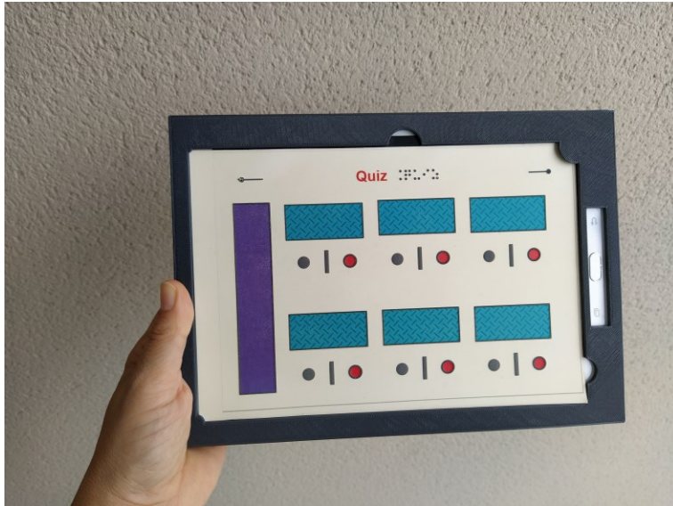
Figure 105. Designed tablet case for fixing raised-line graphics.
