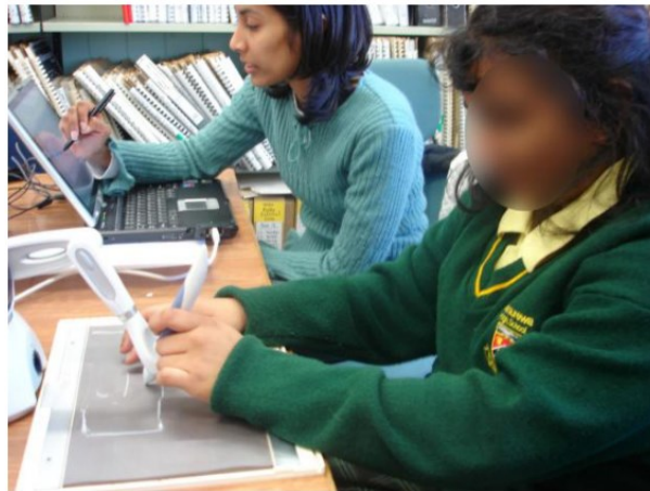
Figure 40. The system McSig [104]. The teacher on the left draws on a Tablet PC to create a shape and the student on the right can feel, explore and be moved around the shape.
