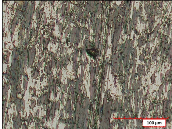
Figure 10: Disc track observed on optical microscopy when testing at 1.24 MPa of pressure and 25.0 m/s of speed (PV = 31 MPa.m/s)
