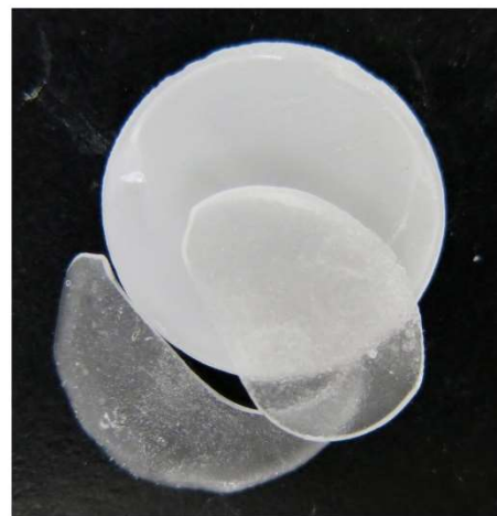
Fig. 1 – Fractured VM7 sample.
