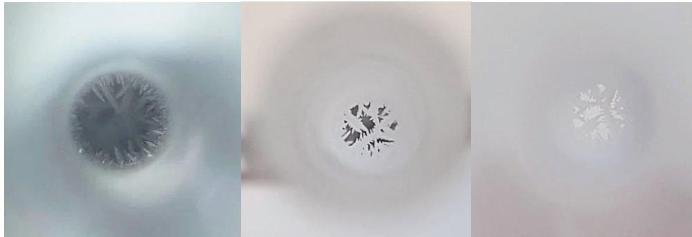
Figure II-13. Pictures of NH<sub>3</sub>NO<sub>3</sub> ammonium nitrate solidified on inner tube walls during Fast SCR conditions.
