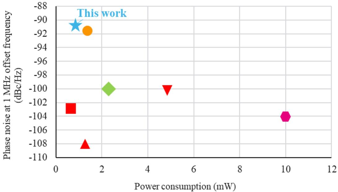
Figure 6.12: State-of-the-Art comparison: phase noise performance at 1 MHz offset frequency from the carrier versus power consumption.
