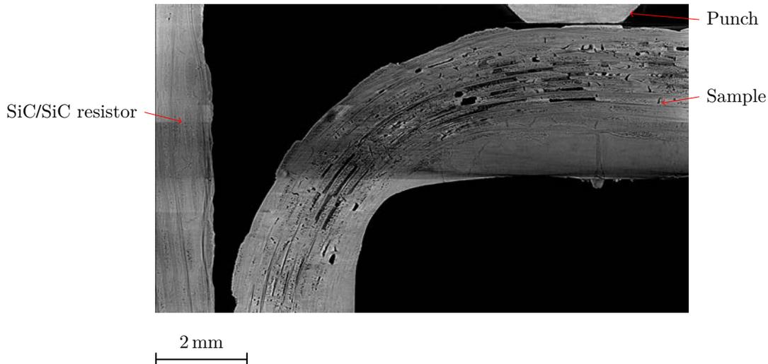
Figure 5.8 – Tomography of the sample where the beam hardening is noticeable: the part of the sample where the length crossed by the X-ray is higher appears darker.
