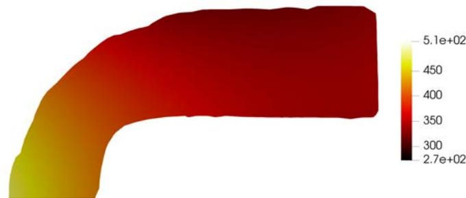
Figure 5.16 – Temperature field in the sample, cut at the middle plane (°C).
