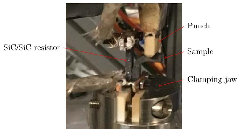
Figure 5.3 – Thermo-mechanical loading of the sample.
