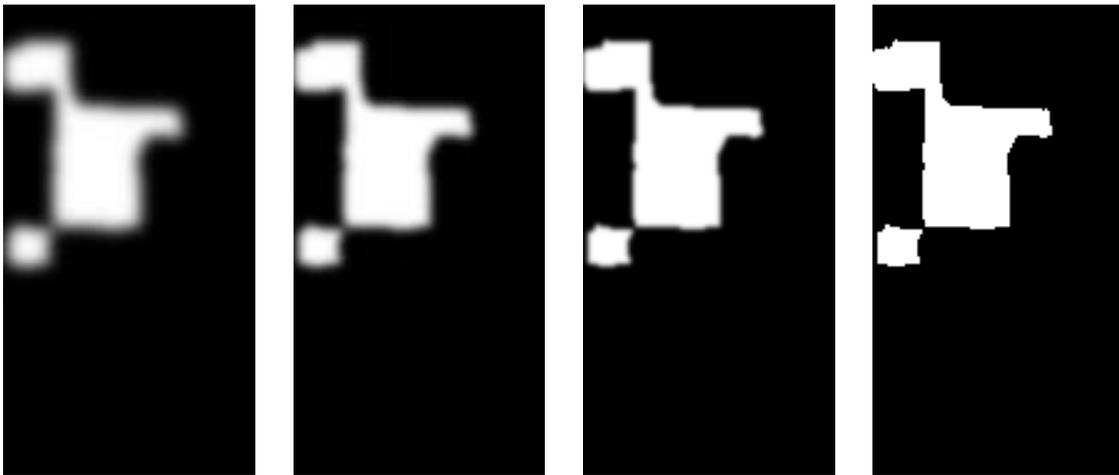
Figure 3.17 – Blurred binarized thermograms used in the pyramidal approach,  $\sigma = [3, 2, 1, 0$  px] from left to right.
