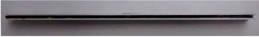
Figure 2.13: Rubber and aluminum sandwich-like structure for the experimental determination of the viscoelastic parameters
