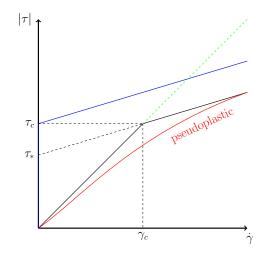
Figure 6.3: Simplified shear-thinning model. We consider a piecewise linear approximation (in black) of the "theoretical" pseudoplastic law (in red). Parameters  $\tau_*$  and  $\tau_c$  are defined by (6.2.10). The blue curve is the Bingham limit:  $\nu_B \to +\infty$ ,  $\gamma_c \to 0$  with  $\gamma_c \nu_B = \tau_c$ . The green dashed line is the pure Newtonian limit  $\nu_B \to \nu$ .
