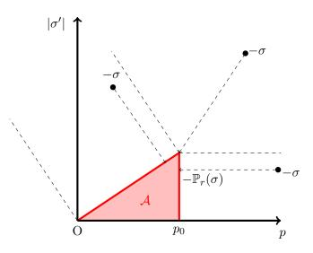
Figure 2.3: Set  $\mathcal{A}$  in the Drucker-dilatant model with 4 possible cases of projections.
