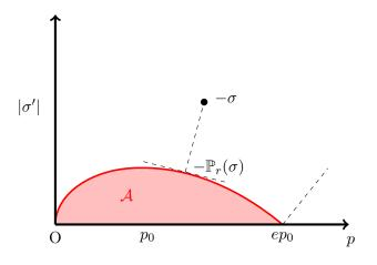
Figure 2.4: Set  $\mathcal{A}$  in the logarithmic model, and orthogonal projection.
