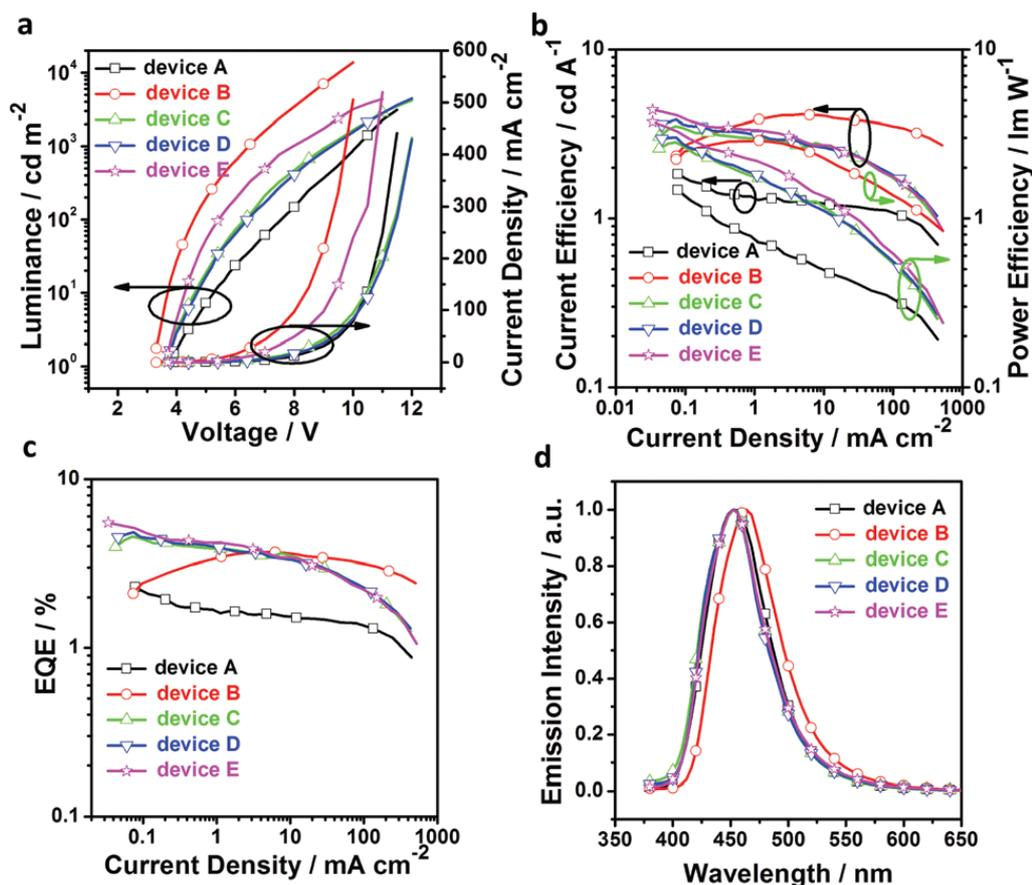
**Figure 20.** *J-V-L characteristics (a), power and current efficiency (b), EQE vs current density plot (c) and EL spectra (d) for OLEDs fabricated with compounds 35 and 36.<sup>[80]</sup>*
