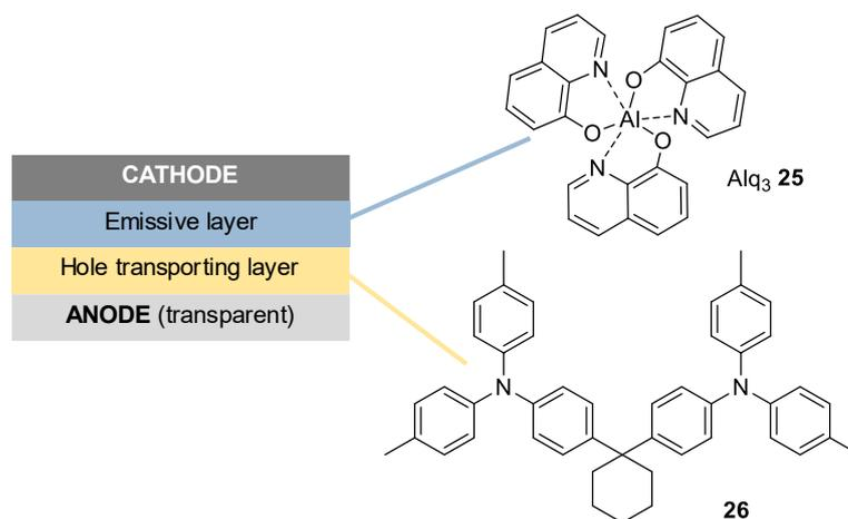
**Figure 14.** Composition and structure of the very first OLED device by Tang and Van Slyke.<sup>[65]</sup>
