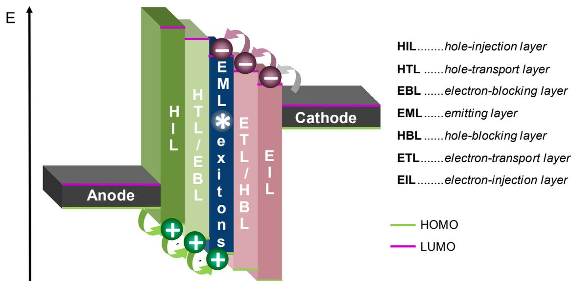
*Figure 16.* General architecture of an OLED device.
