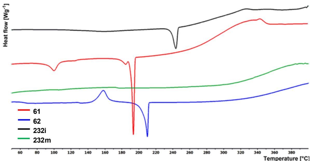
Figure 54. DSC thermograms of compounds **61**, **62**, **232i** and **232m**.
