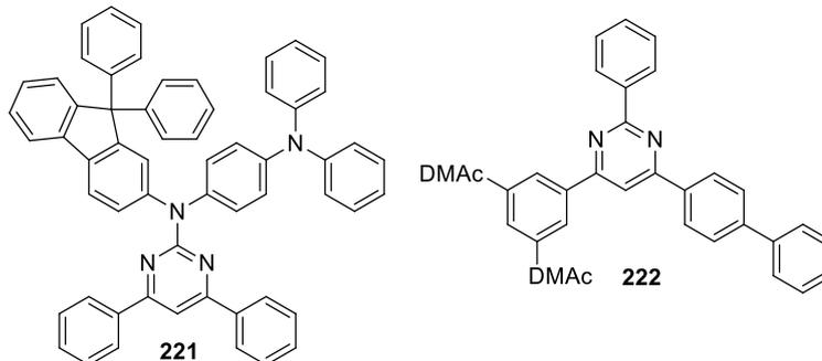
**Figure 50.** Miscellaneous pyrimidine-based host materials **221** and **222**.
