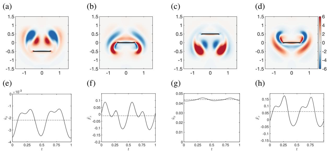
Figure 3.14: Leading and secondary unstable synchronous Floquet mode for  $\beta = 35$ : (a-d) Vorticity contours for four equally spaced time instants along a flapping period. Foil horizontal (e,g) velocity and (f,h) force respectively for the leading and secondary unstable multipliers. Mean force and speed in all figures represented by a dashed line.
