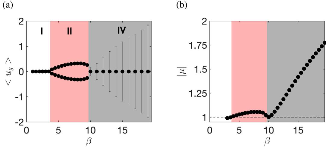
Figure 2.21: Evolution of the (a) time-averaged horizontal velocity and (b) leading Floquet multiplier absolute value of an elliptical foil of minor/major axis aspect ratio  $h = 0.1$  with control parameters  $A = 0.5$  and  $\rho = 32$ . In (a) - resp. (b) - white, red and grey background colors identify symmetric non-propulsive, unidirectional propulsive and back & forth regimes - resp. stable, synchronous unstable and asynchronous unstable multipliers.
