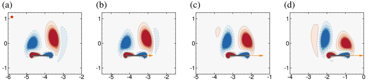
Figure 2.7: Back & Forth solution for  $\beta = 13$ : (a-d) Vorticity contours of the time instants represented in figure 2.6(e) by filled red dots. An orange arrow indicates the horizontal velocity of these time instants. These time instants are equally spaced of 3 flapping periods.
