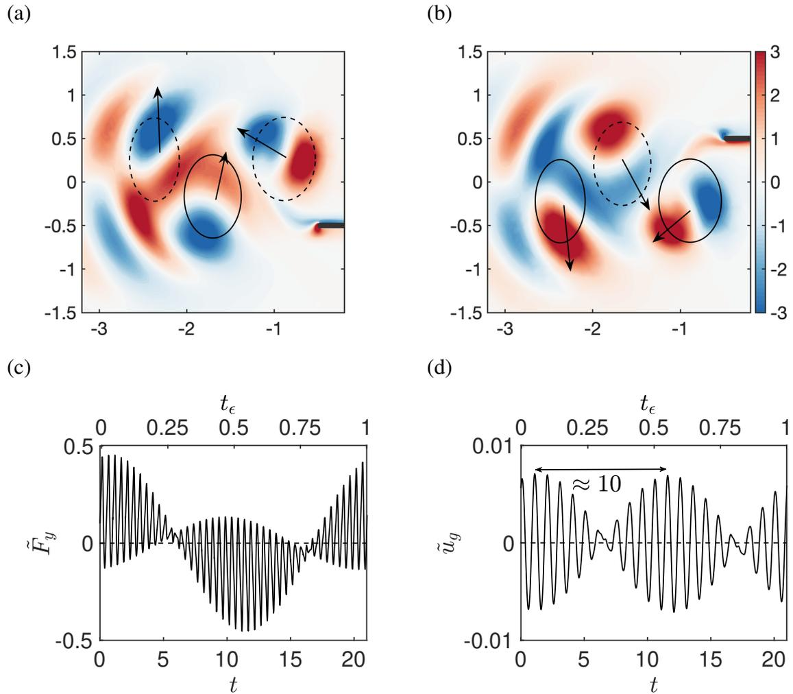
Figure 3.9: Temporal evolution of the quasi-periodic perturbation  $\tilde{\mathbf{q}}$  for  $\beta = 22.43$ : (a,b) Perturbation (colors) and base-flow (with positive values in solid and negative in dashed lines) vorticity for  $t_\epsilon = 0$  and  $t_\epsilon = 0.5$  of the slow period  $T_\epsilon = 1/f' = 23$ . (c) Vertical force and (d) horizontal velocity. The time-averaged value of these quantities along the slow period is shown in (c,d) by a dashed line.
