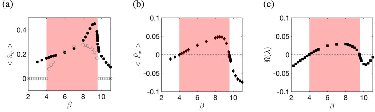
Figure 2.14: Time-averaged horizontal (a) velocity and (b) force for the synchronous Floquet mode as a function of  $\beta$ . (c) Real part of the Floquet exponent. In (a) the mean horizontal speed obtained with nonlinear simulations is represented with empty grey circles for comparison.
