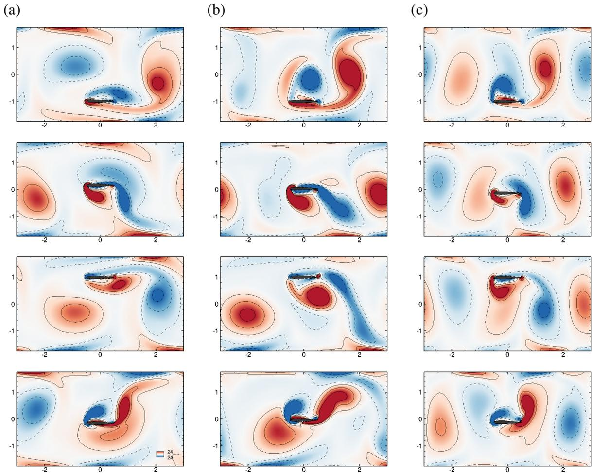
Figure 6.5: Four equally spaced along a flapping period flow vorticity contours of the self-propelled infinite array of flapping wings. For  $\beta = 15$  (a) fast solution with constructive trailing edge wake interaction, (b) unstable intermediary solution and (c) slow solution with constructive leading edge wake interaction. Fixed parameters are  $\rho = 10$ ,  $A = 1$ ,  $L = 6$ ,  $H = 3.5$ .
