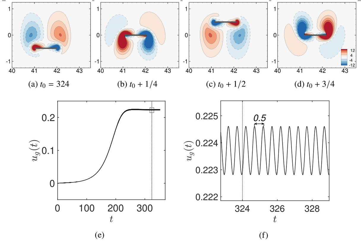
Figure 2.4: Unidirectional propulsive solution for  $\beta = 6$ : (a-d) Vorticity flow field along a flapping period. Time evolution of the horizontal velocity  $u_g$  (initially equal to zero) (e) over the whole simulated time and (f) restricted to time window indicated by the rectangle in (e). The instant  $t_0$  is depicted with a vertical line in (e) and (f). The period of the horizontal velocity is 0.5, half the vertical flapping period 1.
