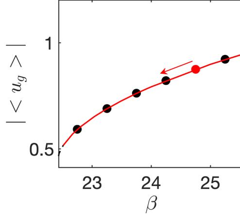
Figure 1.12: Validation of the pseudo arc-length continuation method (solid red line) with respect to results of unsteady nonlinear simulations (black filled circles) for  $23 \leq \beta \leq 26$ . The initial solution and tangent given to the algorithm are represented by a red filled circle and arrow.
