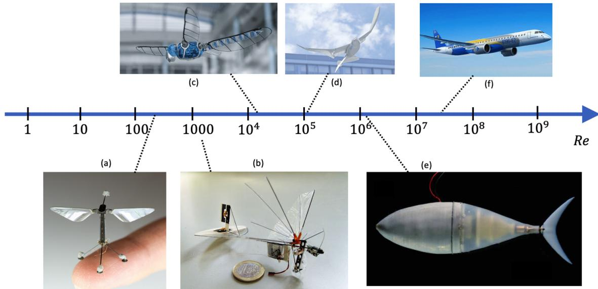
Figure 2: Average Reynolds number range of mankind flying (and one swimming) devices (Calculated based on the references). Flapping wing propulsion micro aerial vehicles (FWMAV) such as (a) Robobee (Chen et al. 2019), (b) Delfly Micro (Deng, Percin, and Van Oudheusden 2015), (c) Festo BionicOpter (Gaissert et al. 2011), (d) Festo SmartBird (Send et al. 2012), the tuna inspired swimming robot (e) Tunabot (Zhu et al. 2019) and (f) commercial jets (Embraer E195-E2).
