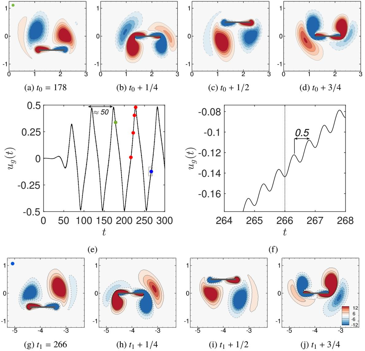
Figure 2.6: Back & Forth solution for  $\beta = 13$ : (a-d) and (g-j) Vorticity contours for a flapping period – starting from different time instants in (a) and (g). (e-f) Horizontal speed  $u_g$  time evolution with dotted rectangle close-up in (f). Instants (a) and (g) are indicated by filled green and blue dots in (e). Long and small periods of  $u_g(t)$  are respectively indicated in (e) and (f).
