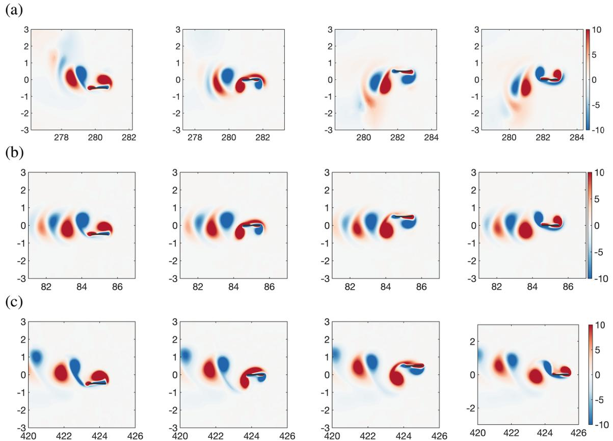
Figure 3.1: Vorticity snapshots for (a) Deviated Quasi- Periodic Wake (DQPW,  $\beta = 21$ ), (b) Symmetric Periodic Wake (SPW,  $\beta = 23$ ) and (c) Deviated Periodic Wake (DPW,  $\beta = 30$ ) propulsive solutions. The time instants are separated by 4.25 in (a) and by 0.25 in (b,c). The initial instants (shown in the next figure) correspond to the position  $y_g = -0.5$ .
