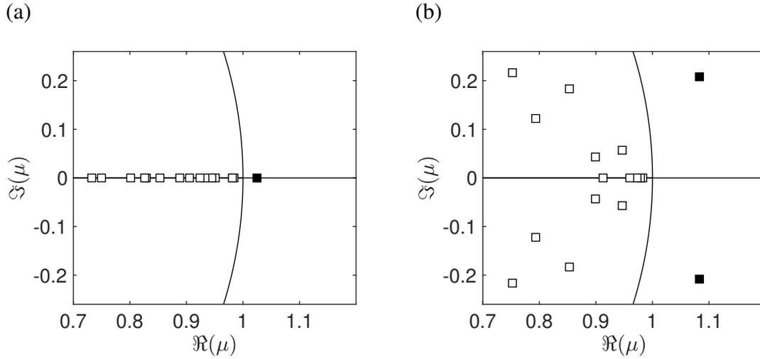
Figure 1.13: Spectra of the Floquet multipliers for two Stokes numbers obtained through fluid-solid Floquet stability analysis. Spectra for (a)  $\beta = 6$  presenting one unstable synchronous multiplier (filled square) and (b)  $\beta = 13$  presenting a pair of complex conjugate unstable asynchronous multipliers. Other control parameters are  $A = 0.5$ ,  $\rho = 100$  and  $h = 0.05$ .
