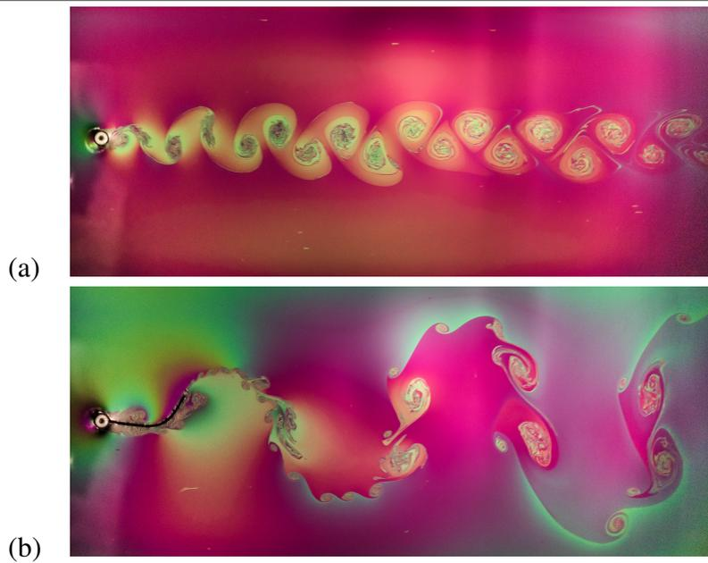
Figure 5: Examples of purely hydrodynamic and coupled fluid solid instabilities in a soap-film flow experiment (Pfister et al. 2020). (a) Von-Kármán vortex wake behind a fixed circular cylinder. (b) Interaction of this vortex shedding with a flexible filament (a silk thread in the experiment) attached behind the cylinder. Incoming flow is oriented towards the right.
