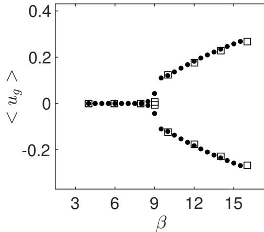
Figure 2.20: Validation of the nonlinear solver. Time-averaged horizontal velocity of the foil as a function of the Stokes number  $\beta$ . Results of the numerical algorithm described in 2.5 (filled dots) are compared to results (empty squares) extracted from figure 13 ( *clamped* case) in Spagnolie et al. (2010).
