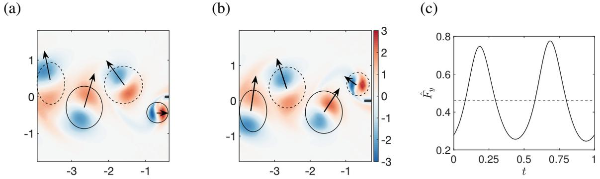
Figure 3.7: Unstable synchronous mode for  $\beta = 30$ : (a,b) perturbation vorticity contours for  $t = 0.25$  and  $t = 0.75$  and base flow positive (resp. negative) vortex contours represented by solid (resp. dashed) lines. Arrows indicate the core displacement of the base-flow vortex due to the perturbation. (c) Vertical force acting on the foil with its time-averaged value represented by a dashed line.
