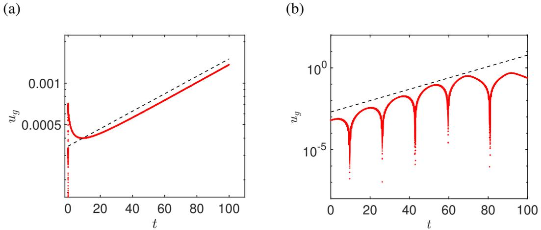
Figure 1.15: Comparison of the growth rate of the horizontal velocity  $u_g$  in unsteady nonlinear simulations with the growth (figure 1.13) predicted by the Floquet multipliers (dashed line) for two Stokes (a)  $\beta = 6$  and (b)  $\beta = 13$ . Other control parameters are  $A = 0.5$ ,  $\rho = 100$  and  $h = 0.05$ .
