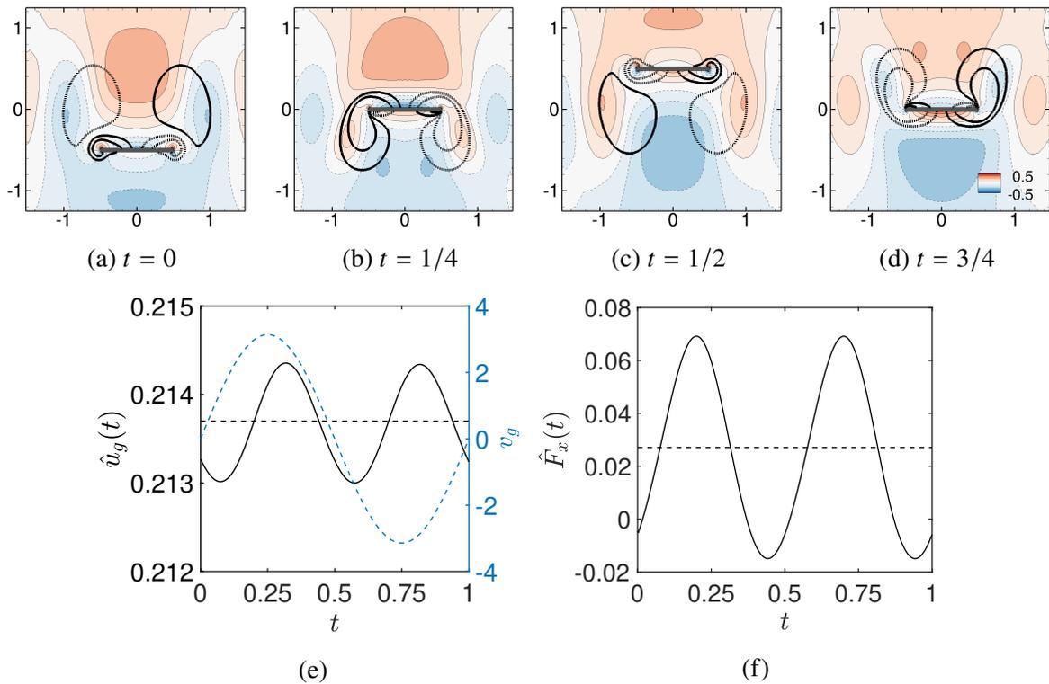
Figure 2.13: Unstable synchronous Floquet mode for  $\beta = 6$ : (a-d) Vorticity contours for a flapping period (base flow positive (resp. negative) values represented by solid (resp. dashed) lines). (e) Foil horizontal speed and (f) force. Time-averaged value along a flapping period of both values is represented by a dashed line in (e,f). In (e) the vertical speed  $v_g$  of the base-flow (light blue dashed line) is represented in the right axis.
