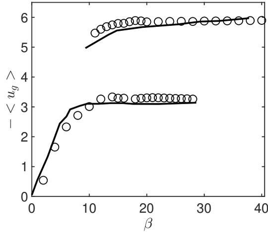
Figure 5.8: (a) Validation between the present numerical method (open circles) and the numerical results of Becker et al. (2015) (solid line). Fixed parameters are  $\rho = 10$ ,  $A = 1$ ,  $H = 3.5$  and  $L = 6$ .
