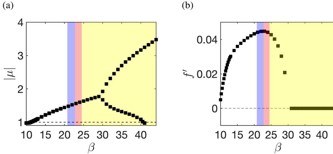
Figure 3.13: Fluid-solid stability analysis of non-propulsive solutions. (a) Absolute value and (b) frequency of the leading Floquet multiplier as a function of the Stokes number  $\beta$ . For comparison, the background colors violet, red and yellow indicate regions presenting quasi-periodic, symmetric periodic wake and deviated wake propulsive solutions, as identified in §3.2.2
