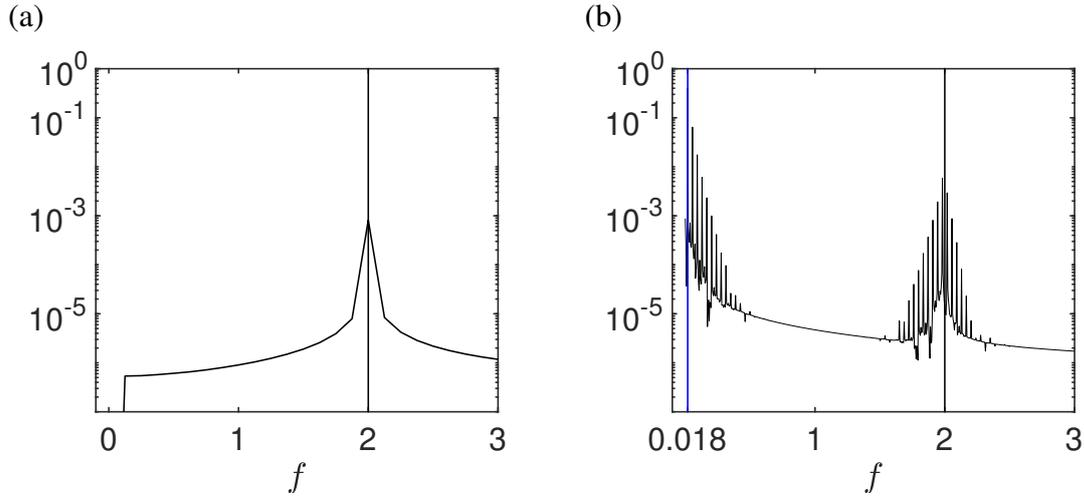
Figure 2.5: Frequency spectra of the horizontal foil speed for (a) the periodic unidirectional propulsive solution ( $\beta = 6$ ) and (b) the quasi-periodic back & forth propulsive solution ( $\beta = 13$ ). The fundamental frequency of the horizontal speed (vertical black lines) is twice the vertical flapping frequency. The low frequency of the quasi-periodic solution (figure 2.6-e) is identified by the blue line.
