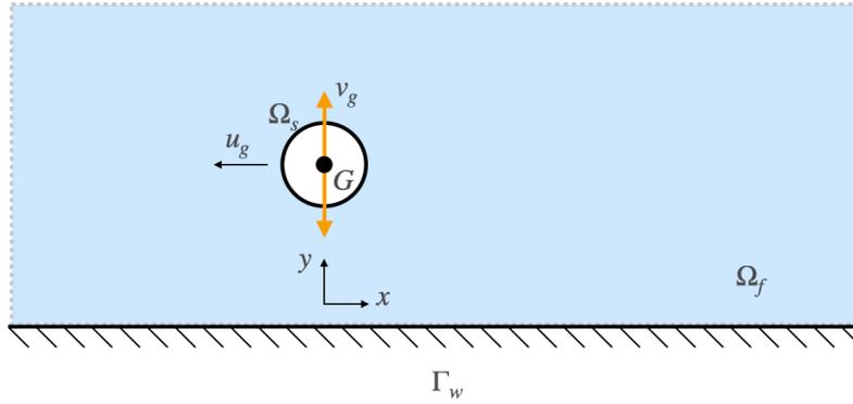
Figure 5.2: Arbitrary configuration of a rigid solid body  $\Omega_s$  interacting with a surrounding fluid  $\Omega_f$  nearby a solid wall  $\Gamma_w$ . The body horizontal  $u_g$ , vertical velocity  $v_g$  flapping movement (orange arrow), center of gravity  $G$  and the frame of reference are indicated in the figure.
