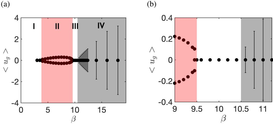
Figure 2.9: Self-propelled regimes for a density ratio  $\rho = 1$ . Background colors are the same as the previous figure. (a) Evolution of the time-averaged (circles) and amplitude (error bars) of the foil horizontal velocity with the Stokes number. (b) Close-up view highlighting the transition between the self-propelled regimes. Other control parameters:  $A = 0.5$  and  $h = 0.05$ .
