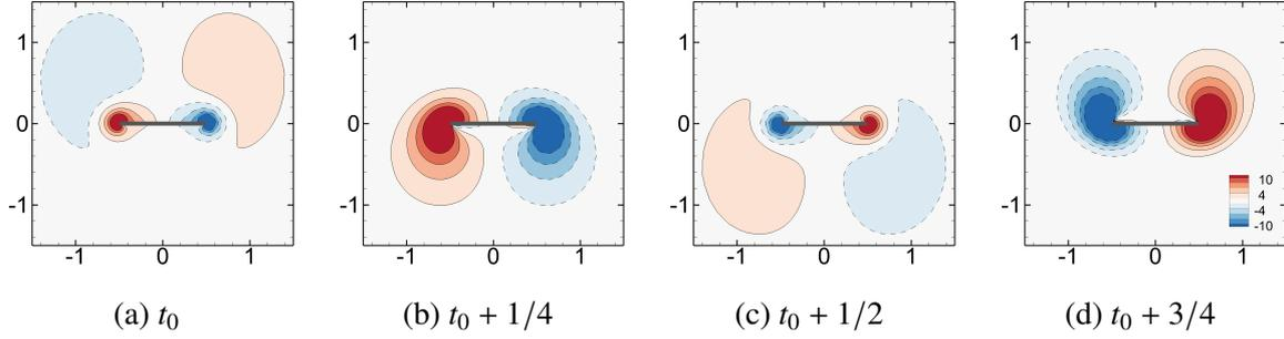
Figure 8: Symmetric solution for  $\beta = 2$ . The vorticity field is depicted in the non-inertial frame of reference  $(x, y)$  (a-d) for four equally-spaced instant of the unitary period. The initial time  $t_0$  corresponds to the lowest vertical position of the foil.
