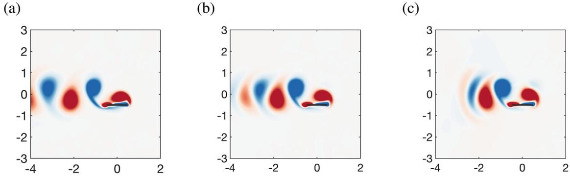
Figure 3.5: Symmetric periodic wake propulsive solutions obtained with the Time Spectral Methods. The three solutions represented are the grey  $\times$  in figure 3.4 progressively decreasing the horizontal speed (a)  $\beta = 30$ , (b)  $\beta = 23.2$  and (c)  $\beta = 23.2$  (inside the saddle branch). The same scale as fig. 3.1 is used for the contours.
