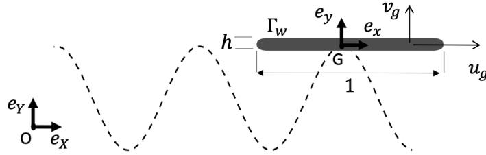
Figure 1.1: Sketch of the foil configuration under sinusoidal vertical motion and horizontal translation with velocity  $\mathbf{u}_g$ . The foil chord (trailing to leading edge) and its thickness, the frames of reference and the solid/fluid interface  $\Gamma_w$  are indicated.
