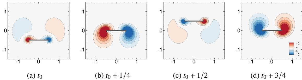
Figure 1.2: Fluid flow (colors) vorticity field and foil flapping movement (grey) depicted in the laboratory frame of reference  $(O, X, Y)$  of Fig. 1.1. (a-d) for four equally-spaced along a flapping period.
