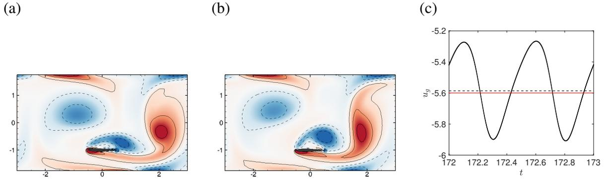
Figure 6.13: Comparison for  $\beta = 15$  between (a) self-propelled and (b) *quasi*-self-propelled solution for  $-\langle u_g \rangle = 5.6$ . (c) Comparison between the unsteady  $u_g$  signal and the self (dashed black line) and *quasi*-self-propelled (red line) time-averaged velocity values. Fixed parameters are  $\rho = 10$ ,  $A = 1$ ,  $L = 6$ ,  $H = 3.5$ .
