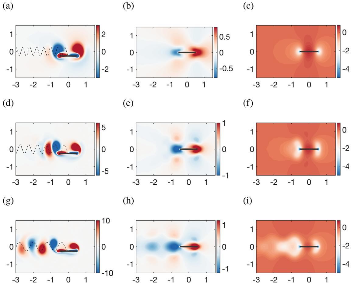
Figure 4.4: (a-c) Diffusion-driven ( $\beta = 14$ ) (d-f) transitional ( $\beta = 39$ ) and (g-i) pressure-driven ( $\beta = 62$ ) self-propelled solutions. (a,d,g) Instantaneous vorticity field, (b,e,h) Time-averaged stream-wise velocity  $u$  field and (c,f,i) the time-averaged pressure  $p$  field. The dashed lines in (a,d,g) correspond to the foil center of mass trajectory.
