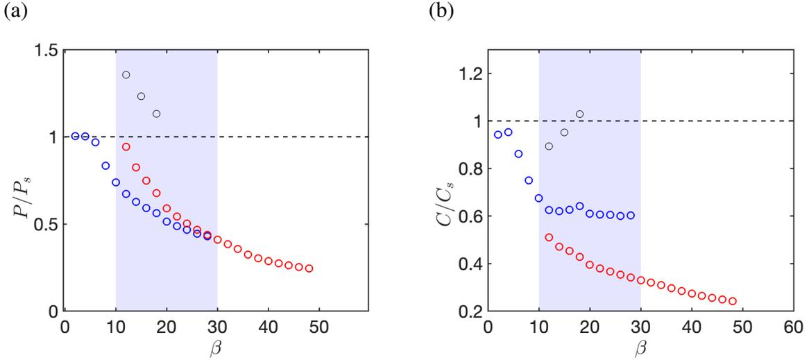
Figure 6.6: Evolution with the Stokes number  $\beta$  of the (a) power input  $P$  and of the (b) cost of transport  $C$  compared to those of single flapping wing ( $P_s$  and  $C_s$ ). Blue, red and black circles identify again slow, fast and unstable solutions. A dashed line highlight in both figures the unitary value when both quantities equal the one of a single wing.
