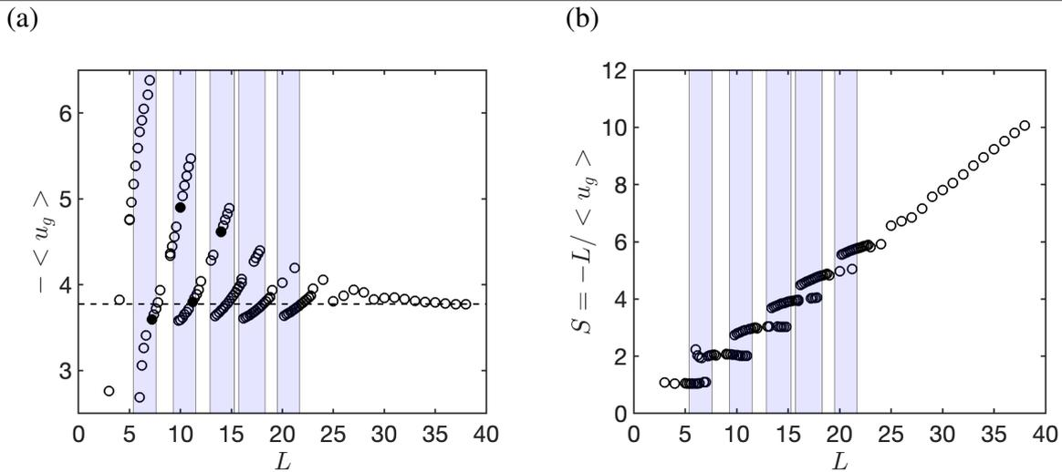
Figure 6.11: (a) Time-averaged horizontal velocity and (b) schooling number  $S = -L / \langle u_g \rangle$  of the self-propelled infinite array evolution with the gap  $L$  between the wings. The light blue background again identify ranges where coexisting solutions are obtained. Contours of the solutions represented by filled circles are in figure 6.12. Other fixed parameters are  $\beta = 15$ ,  $\rho = 10$ ,  $A = 1$ ,  $H = 3.5$ .
