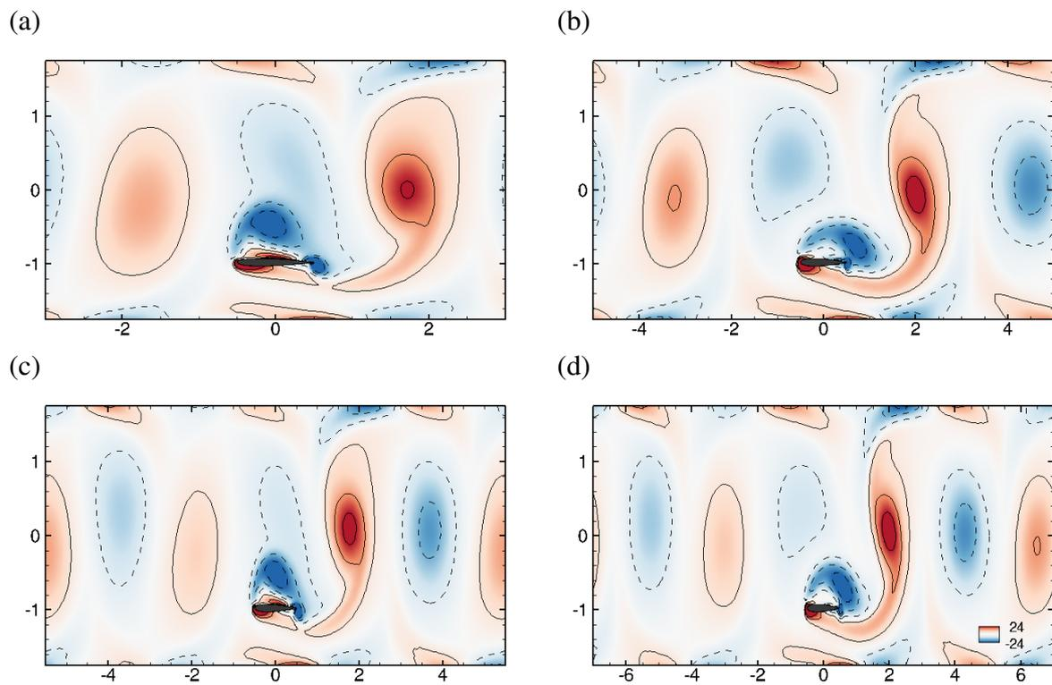
Figure 6.12: Vorticity contours of the self-propelled infinite array of flapping wings for different gaps  $L$  between wings. (a)  $L = 7$  (LE interaction), (b)  $L = 10$  (TE interaction), (c)  $L = 11$  (LE interaction) and (d)  $L = 14$  (TE interaction). Fixed parameters are  $\rho = 10$ ,  $A = 1$ ,  $\beta = 15$ ,  $H = 3.5$ .
