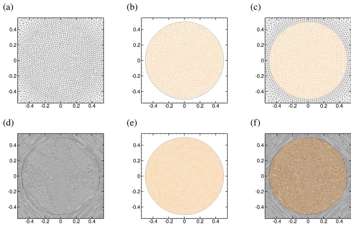
Figure 5.4: Spatial discretization of the (a,d) Fictitious  $\Omega_f \cup \Omega_s$  (black mesh), (b,e) solid  $\Omega_s$  (orange mesh) and (c,f) superposition of the two domains for (a-c) a conforming and (d-f) a non-conforming case.
