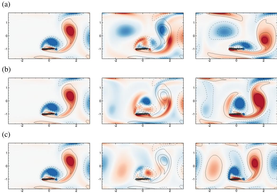
Figure 6.8: Decomposition of the total flow (third column), represented by vorticity contours, in its single wing (first column) and wake interaction (second column) components. For  $\beta = 15$  (a) Fast solution, (b) unstable solution and (c) slow solution. In the second column, we superpose single wing and wake interaction components, that are respectively represented by lines and flooded contours. Other fixed parameters are  $\rho = 10$ ,  $A = 1$ ,  $L = 6$ ,  $H = 3.5$ .
