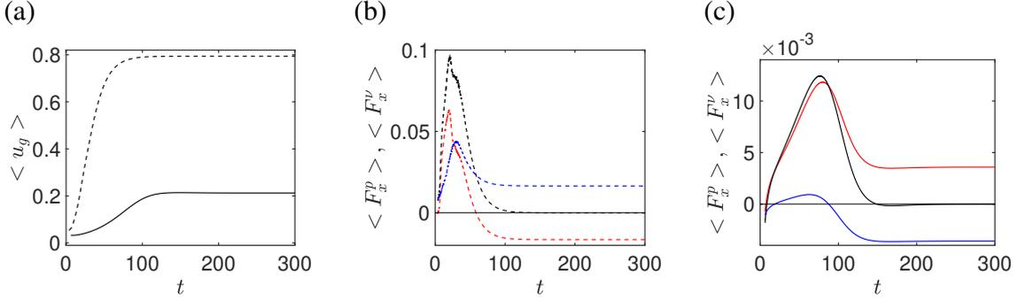
Figure 4.2: Temporal evolution of a diffusion-driven, Stokes number  $\beta = 14$  (solid line), and a pressure-driven,  $\beta = 62$  (dashed line), self-propelled solutions. (a) Horizontal velocity time-averaged over the non-dimensional flapping period  $T = 1$ . (b,c) Time-averaged pressure (blue) and viscous (red) components of the horizontal force (black). Parameters:  $A = 0.25$ ,  $\rho = 100$  and  $h = 0.05$ .
