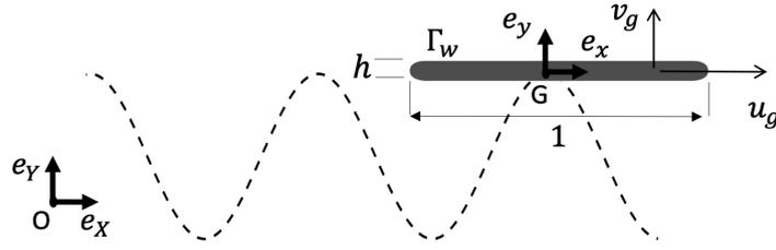
Figure 2.1: Sketch of the foil configuration under sinusoidal vertical motion and horizontal translation with velocity  $\mathbf{u}_g$ . The foil chord (trailing to leading edge) and its thickness, the frames of reference and the solid/fluid interface  $\Gamma_w$  are indicated.
