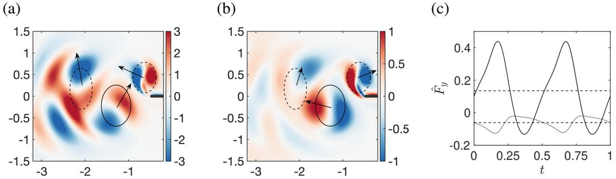
Figure 3.8: Unstable asynchronous mode for  $\beta = 22.43$ : perturbation vorticity contours of the (a) real part and (b) imaginary part for  $t = 0.75$ . Solid and dashed superposed thick lines represent positive and negative values of the base-flow vorticity. Arrows indicate the core displacement of the base-flow vortex due to the perturbation. (c) Real (solid line) and imaginary (dotted line) parts of the vertical force where a dashed line indicate its time-averaged value.
