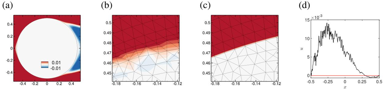
Figure 5.5: (a) Large and close-up (b,c) view of the stream-wise velocity on a cylinder surface for  $Re = 40$  over the fictitious domain. (b) P1 and (c) P2 discretization of the distributed Lagrange multipliers. The fictitious and solid domain are conforming (meshes shown in figure 5.4(a-c)). (d) Value of the horizontal velocity on the cylinder wall upper part  $y \geq 0$ .
