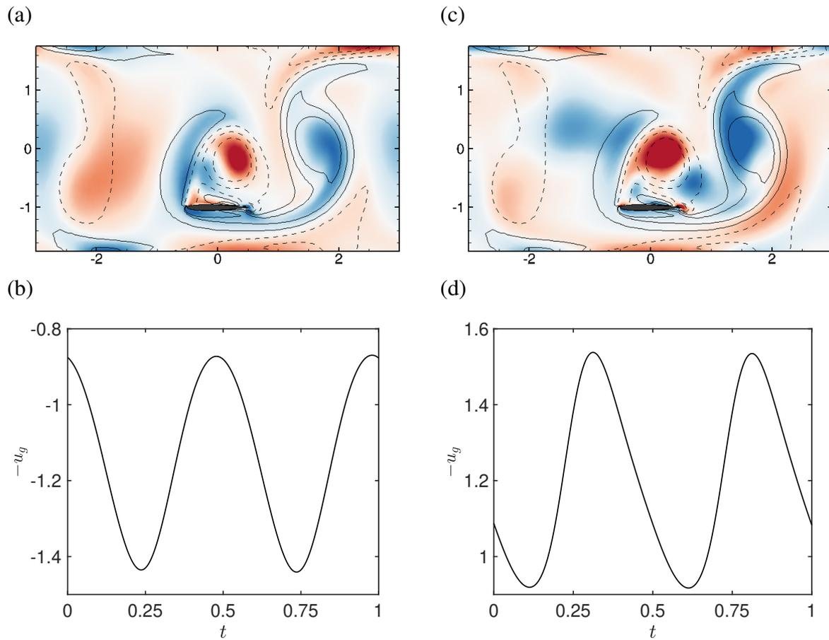
Figure 6.10: Nonlinear perturbation of the unstable *quasi*-self-propelled solution for  $\beta = 15$ : flow vorticity  $\omega''_z$  and horizontal velocity  $u''_g$  periodic evolution leading towards the (a,c) fast and (b,d) slow solutions. In (a,b) the middle unstable solution and the nonlinear perturbation are superposed, respectively represented by lines and flooded contours. Fixed parameters are  $\rho = 10$ ,  $A = 1$ ,  $L = 6$ ,  $H = 3.5$ .
