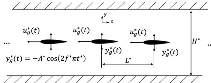
Figure 6.1: Configuration studied: (a) by Becker et al. (2015) and (b) rolled out infinite array used in this study. The system of axis  $(e_x, e_y)$  that follows the foil center of gravity  $g$ , the heaving motion  $y_g^*(t)$ , the horizontal velocity  $u_g^*(t)$ , the fixed gap between wings  $L^*$  and the height channel  $H^*$  are indicated in (b).
