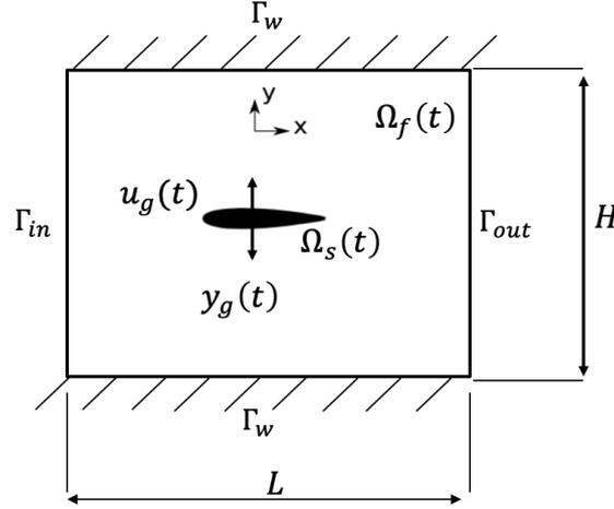
Figure 6.2: Simplification of the infinite array to a single wing in a periodic domain. Inflow ( $\Gamma_{in}$ ), outflow ( $\Gamma_{out}$ ), wall ( $\Gamma_w$ ) boundaries, fluid ( $\Omega_f(t)$ ) and solid domain ( $\Omega_s(t)$ ) are identified in the figure.
