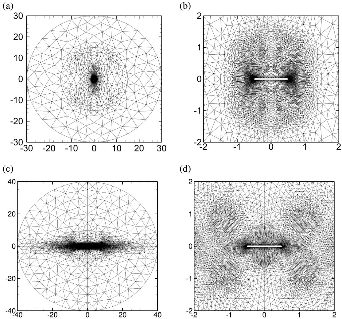
Figure 1.4: (a,c) Far and (b,d) close-up view of the computation domain and a typical adapted mesh used for the numerical simulations of a self-propelled rectangular foil of  $A = 0.5$  and (a,b)  $\beta \leq 20$  and (c,d)  $\beta > 20$ .
