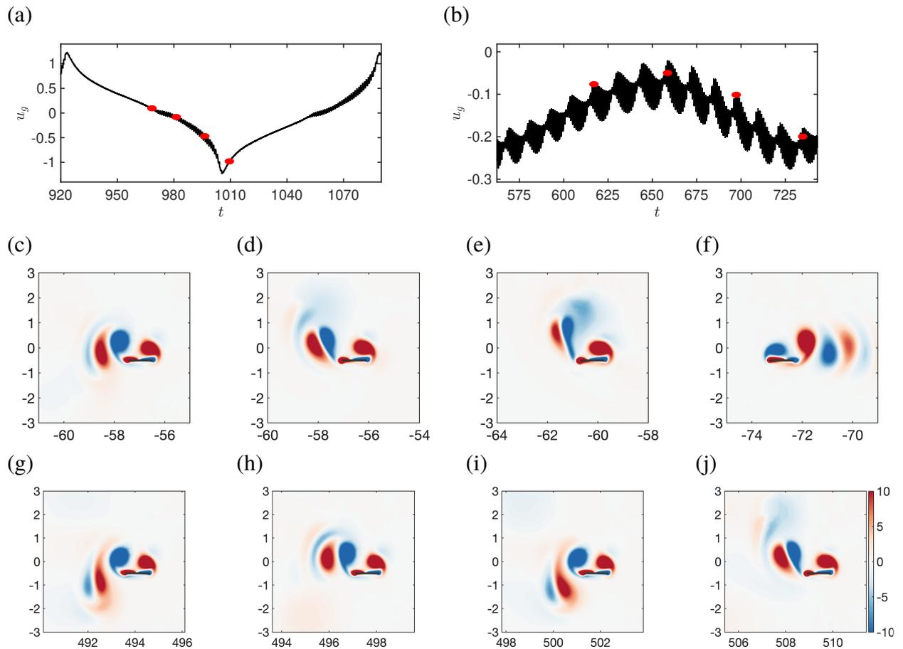
Figure 3.11: Back & Forth solution,  $\beta = 19$  - (a) and (c-f), and transition DQPW solution,  $\beta = 20.25$  - (b) and (g-j). (a,b) Horizontal speed time signals with red filled circles showing the equidistant time instants of (c-f) and (g-j) where the vorticity contours are presented. Images are presented in different horizontal positions.
