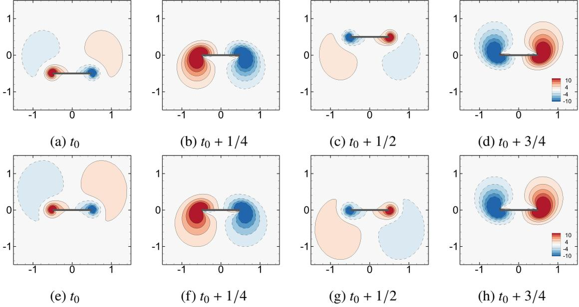
Figure 2.3: Symmetric solution for  $\beta = 2$ . The vorticity field is depicted in the laboratory frame of reference  $(X, Y)$  (a-d) and in the non-inertial frame of reference  $(x, y)$  (e-h) for four equally-spaced instant of the unitary period. The initial time  $t_0$  corresponds to the lowest vertical position of the foil.
