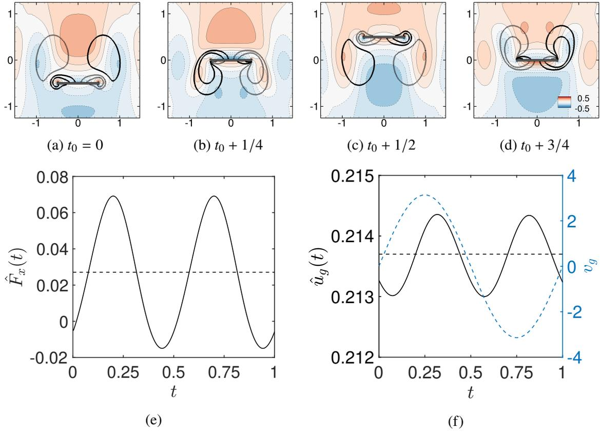
Figure 1.14: Floquet mode obtained with the linear solver a self-propelled wing (fixed parameters  $A = 0.5$ ,  $\rho = 100$  and  $h = 0.05$ ) for  $\beta = 6$ : (a-d) Vorticity contours for a flapping period (base flow represented by thick lines). (e) Horizontal force (black) acting on the solid, with pressure and viscous components in blue and red respectively, and (f) horizontal velocity. Mean force and velocity in both figures with dashed line.
