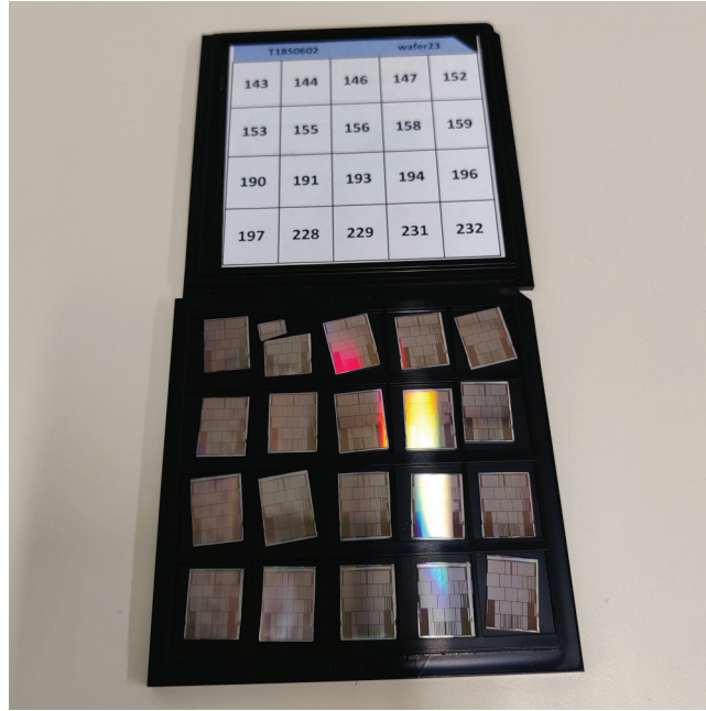
Figure 2.9 – Wafer dicing. The 300mm wafer is cut into dies. Each die contains many samples of different geometries serving different purposes. A wafer map helps identifying the dies numbers depending on their positions in the said wafer. A piece of the second die (top left) containing a desired sample has been cut.
