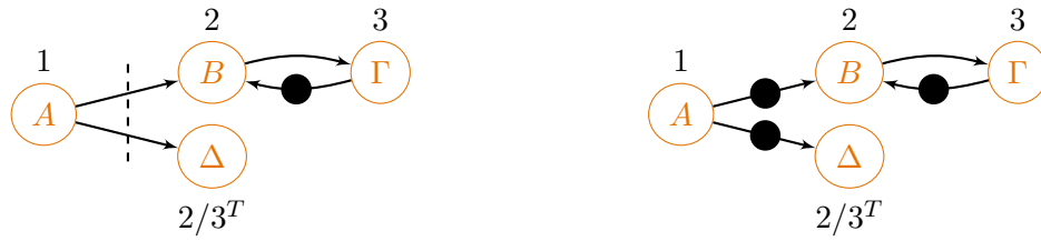
(a) Graph example annotated with ASAP and ALAP topological orderings. ALAP ordering is specified with T , only if different from ASAP. (b) Same graph with pipeline delays added on the cut represented with a dashed line on 4.1a.
