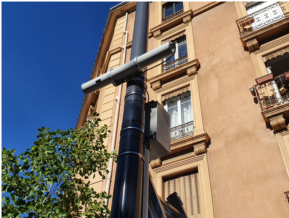
Figure 5.4: Example of a radar sensor for the measurement of road flow. Courtesy: Karrus.
