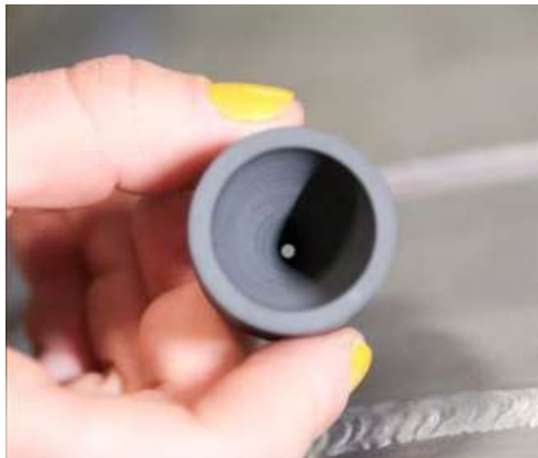
Figure 2.4: Manufactured small dimensional, optimised Laval contoured nozzle (Photo credits: Julien Le Bonheur)
