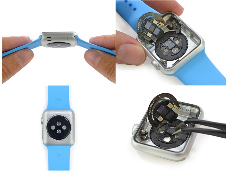
Figure 1.7 – Illustration of the Apple Watch with sensors perfectly integrated inside the back of the watch structure [iFixit].
