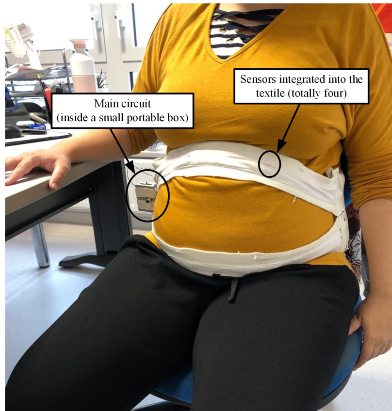
Figure 2.5 – An overall picture of the final intelligent garment prototype integrating the sensors and the main circuit (invisible, inside that small size box).
