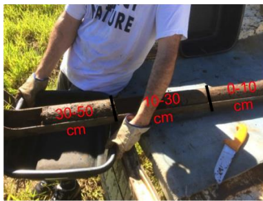
Photo 6. Root sampling (automatic auger and the positioning of soil cores above, soil core and root liberation from soil below).
