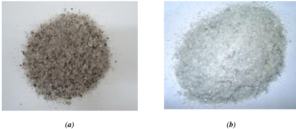
Figure 1.5 Examples of glass waste used as fine aggregates in concrete (a) (Kim et al., 2018) and (b) (Ismail and AL-Hashmi, 2009)
