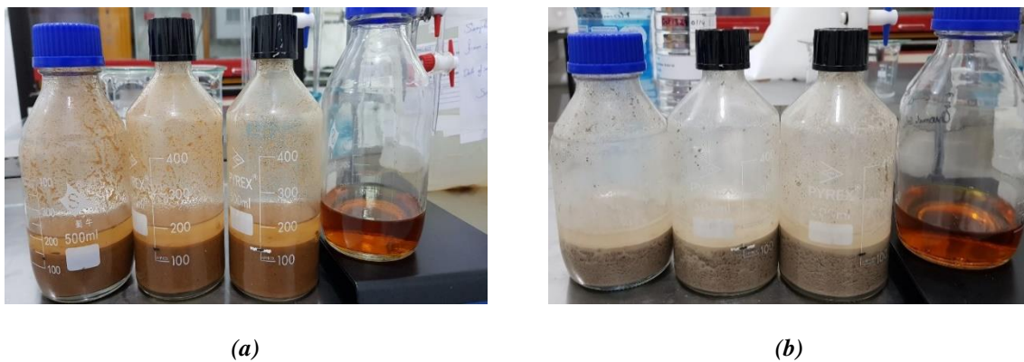
Figure II.14 Organic impurities detection for fine aggregates: (a) natural sand and (b) crushed sand
