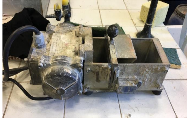
Figure III.4 The apparatus used for the flow time test
