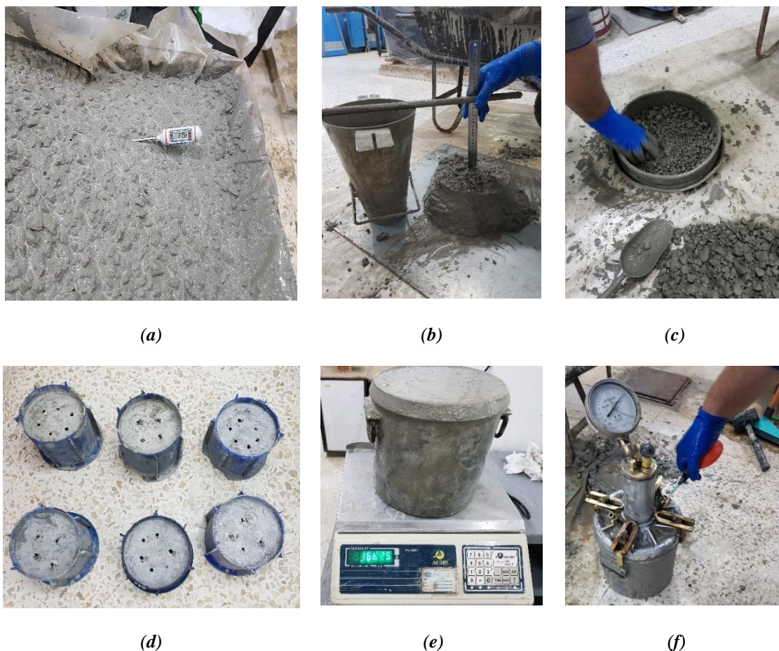
Figure III.12 Illustrations of the tests conducted on the concrete mixes at fresh state: (a) Temperature; (b) Slump and slump retention; (c-d) Setting time; (e) Density; and (f): Air content
