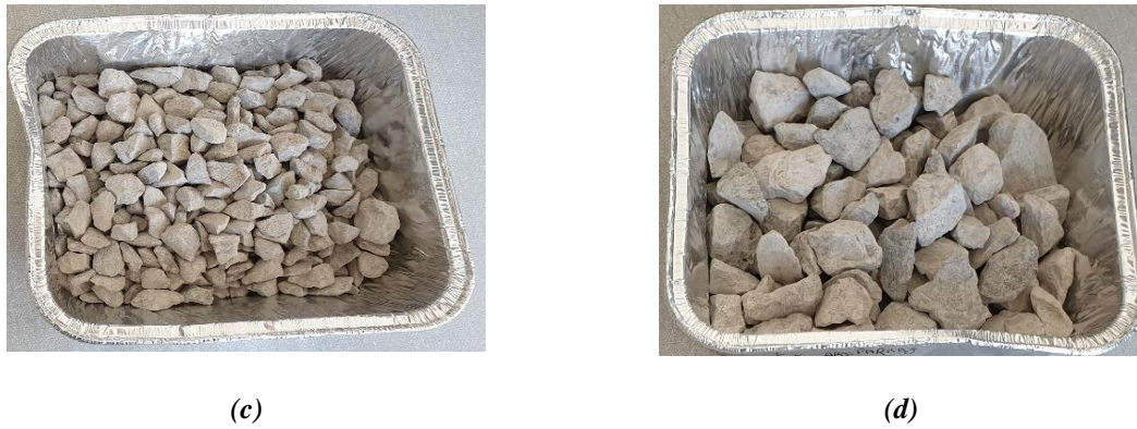
Figure II.1 Simple observation of (a) natural sand, (b) crushed sand, (c) medium aggregate, and (d) coarse aggregate
