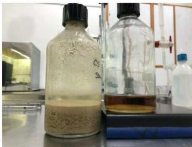
Figure B.2. Comparison of the crushed sand solution (at the left) to the standard color solution (at the right) to detect organic impurities in crushed sand
