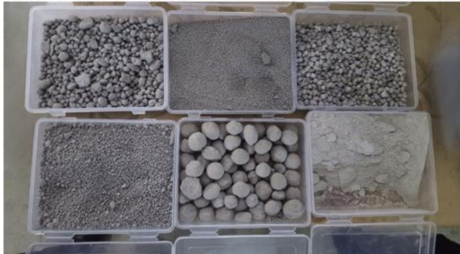
Figure I.9 Different particle sizes of the geopolymer fly ash (Agrawal et al., 2017)
