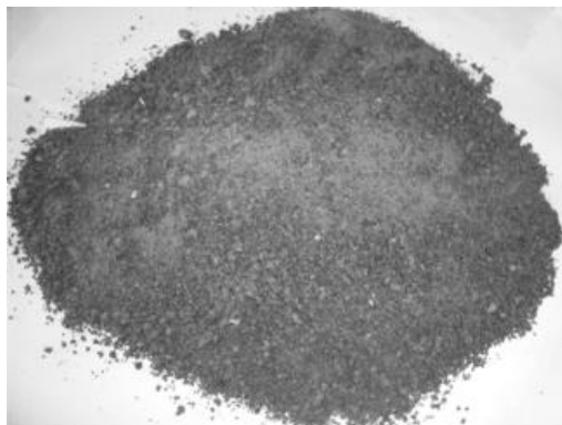
Figure I.11 Ferrochrome slag used as fine aggregate (Panda et al., 2013)
