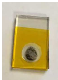
Figure 47. Drop-casting r-Fe@FeOx NPs on an FTO electrode for testing water oxidation catalytic activity at pH 7 and pH 13.
