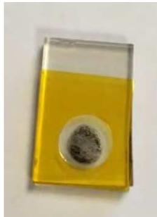
**Figure 47.** Drop-casting *r-Fe@FeOx* NPs on an FTO electrode for testing water oxidation catalytic activity at pH 7 and pH 13.
