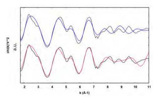
**Figure 34**. Overlap function Chi(k) of **r-Fe@FeOx NPs** (black line) with model 1 (blue line) and model 2 (pink line).
