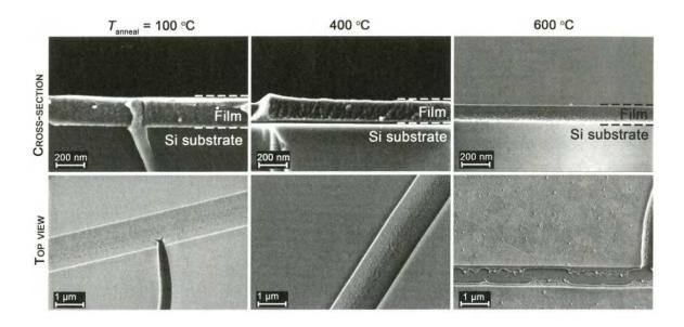
**Figure 2**. SEM cross-section and top-down surface images of amorphous  $Fe_2O_3$  films prepared by PMOD, followed by a 1-hour annealing step in air at  $T = 100^\circ$ ,  $400^\circ$  and  $600^\circ$ [5].
