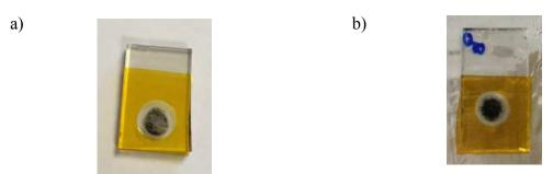
Figure 29. Photograph images of a) r-Fe@FeOx photoanode and b) m-Fe@FeOx@Ru photoanode by drop-casting on FTO electrodes for testing their photocatalytic activity.
