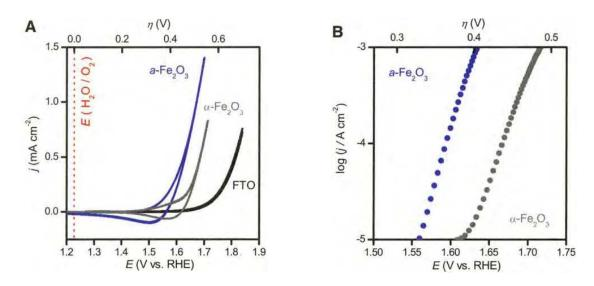
**Figure 3**. A) cyclic voltammograms for films of a-  $Fe_2O_3$  (blue) and hematite (gray), and a blank fluorine-doped tin oxide (FTO) substrate. B) Tafel plot showing the higher catalytic activity of a- $Fe_2O_3$  relative to hematite in 0.1 M KOH[5].
