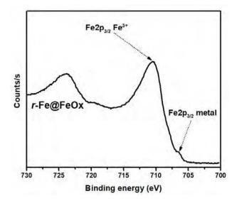
Figure 36. Fe2p XPS spectrum of r-Fe@FeOx NPs
