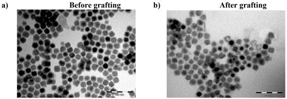
Figure 42. Typical HR-TEM images of a) r-Fe@FeOx NPs (scale bar= 50 nm), and b) r-
