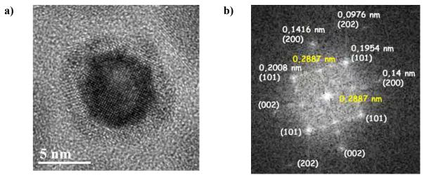
Figure 27. a) typical HR-TEM image of one a-Fe@FeOx NP, and b) corresponding FFT calculation.
