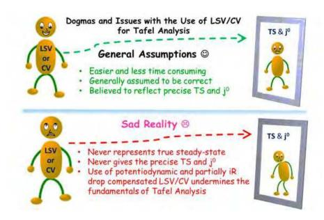
**Scheme 4**. Graphical sketch advocating against the use of dynamic LSV/CV responses for deriving Tafel plots. TS and j<sup>0</sup> denote Tafel slope and exchange current density, respectively[52].
