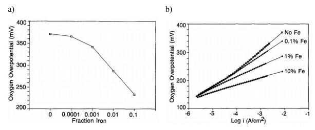
**Figure 2**. Effect of coprecipitated iron a) on the overpotential (results from steady-state polarization measurements at  $8 \text{ mA/cm}^2$ ) and b) on the Tafel plots (results from open-circuit decay measurements) for OER at nickel oxide thin film electrodes[8].
