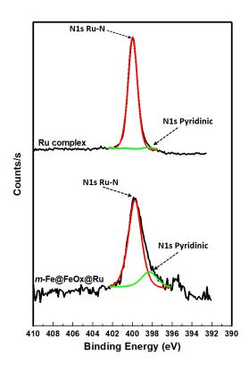
Figure 26. XPS spectra of the free Ru complex (top), and m-Fe@FeOx@Ru NPs (bottom) in the N1s region.
