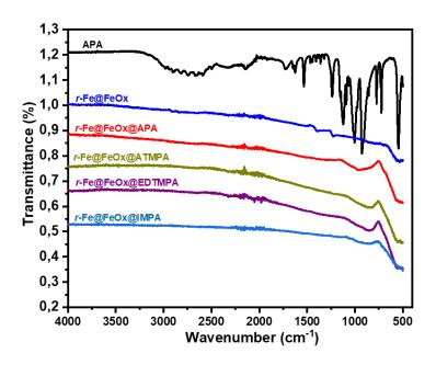
Figure 45. FT-IR of r-Fe@FeOx@APA NPs (red curve), r-Fe@FeOx@ATMPA NPs (dark yellow curve), r-Fe@FeOx@EDTMPA NPs (purple curve), r-Fe@FeOx@IMPA NPs (cyan curve) in comparison with pristine r-Fe@FeOx NPs (blue curve), and APA (black curve).
