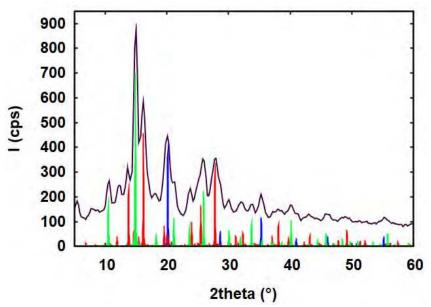
Figure 31. WAXS diagrams of r-Fe@FeOx NPs (black solid line) in comparison with bcc-Fe (PDF-01-071-4648, in blue),  $\gamma$ -Fe<sub>2</sub>O<sub>3</sub> (PDF-01-089-5894, in red) and NH<sub>4</sub>Cl (PDF 96-901-0007, in green) references.
