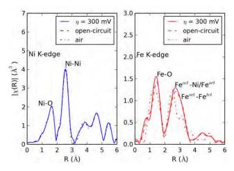
**Figure 8**. Fourrier transform magnitudes of  $k_2$ -weighted EXAFS data for the Ni and Fe K-edges of the 10 at.% Fe mixed Ni-Fe oxide catalyst in air, under open circuit conditions in alkaline electrolyte, and at an overpotential of 300 mV under OER conditions[7].
