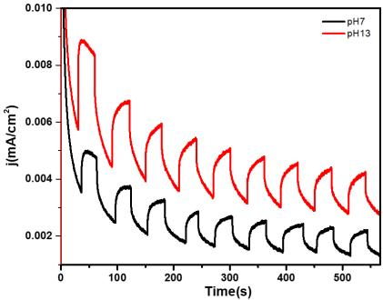
Figure 33. Chopped light measurement at an applied potential 1.0 V vs. RHE of b-Fe@FeO<sub>x</sub>@Ru photoanodes in pH 7 and pH 13 under 1 Sun illumination.
