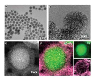
Figure 11. Electron microscopy characterization of NiOx-NiOx/FeOx core-mixed shell NPs A) TEM image overview of the NPs with an average diameter of  $16.8 \pm 2.0$  nm: B) HR-TEM and HAADF-STEM images displaying a representative NP in A which is mostly amorphous; (D) Electron energy loss spectroscopy (EELS) mapping of the NP in C with Ni (green), Fe (pink), and Ni-Fe overlaid maps indicating a NiOx-NiOx/FeOx core-mixed shell morphology. The Ni/Fe atomic ratio of the shell is 0.39:1[18].
