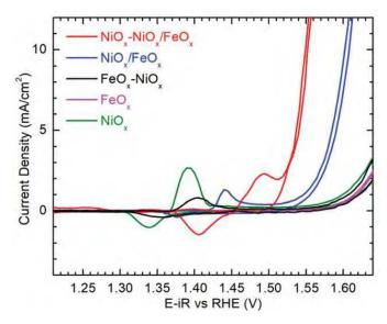
Figure 13. Cyclic voltammograms of the NPs catalysts obtained in 1M KOH at a scan rate of 10 mV.s<sup>-1</sup>: NiOx-NiOx/FeOx core-mixed shell (red), NiOx-FeOx alloy (blue), FeOx-NiOx core-shell (black), FeOx (pink), and NiOx (green)[18].
