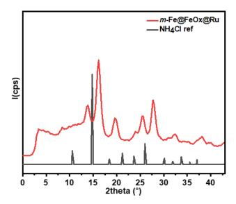
*Figure 22.* WAXS diagram of *m-Fe*@*FeO<sub>x</sub>*@*Ru NPs* in comparison with NH<sub>4</sub>Cl (PDF 96-901-0007).
