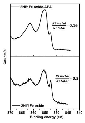
Figure 45. XPS Ni2p spectra of sample 2Ni/1Fe oxide-APA NPs (top) and sample 2Ni/1Fe oxide (bottom)
