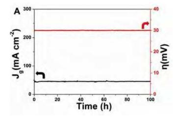
**Figure 17**. The chronoamperometry (CA) of NiFeO-400 NC at the overpotential of 300 mV, and CP curves of NiFeO-400 at geometric current density of 40 mA/cm<sup>2</sup>[19].
