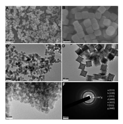
Figure 15. A-B) SEM images of NiFeO-400 NCs under different magnifications: (A) 0.2 μm, (B) 50 nm. (C,D,E) TEM images of NiFeO-400 NCs under different magnifications: (C) 0.2 μm, (D) 50 nm and (E) 10 nm. (F) SAED pattern of NiFeO-400 NCs[19].
