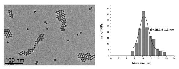
Figure 23. a) TEM images and b) corresponding size histograms of n-Fe@FeOx NPs Fe NPs.
