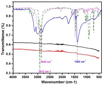
Figure 20. ATR-IR spectrum of Fe NPs (black solid line), n-Fe@FeOx NPs (red solid line) compared to HDA (green dash line), HDA. HCl (pink dot line) and NH<sub>4</sub>Cl reference spectra (blue solid line).
