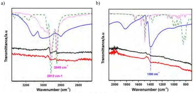
Figure 21. a) Zoom on the vC-H stretching of alkyl chains b) zoom on the triply degenerate vN-H vibrations of NH<sub>4</sub>Cl.
