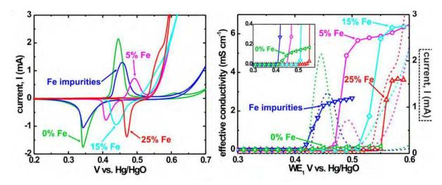
Figure 3. left: CV scan of  $Ni_{1-x}Fe_x(OH)_2/Ni_{1-x}Fe_xOOH$  films deposited on Au/Ti/quartz interdigitated (IDA) electrodes; right: conductivity data (points with solid connecting lines) for the corresponding films. The potential onset of conductivity correlates with the position of the hydroxide/oxyhydroxide oxidation wave shown as dotted lines for each film. The insert shows an enlarged region to make apparent the conductivity turn-on for the rigorously Fe-free film [3].
