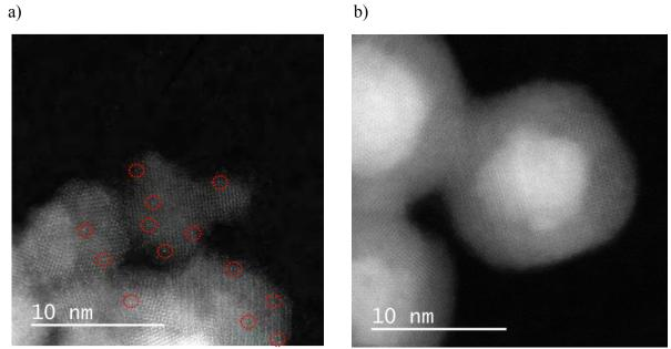
Figure 24. Atomic resolution micrographs obtained by HR-HAADF-STEM of a) m-Fe@FeO<sub>x</sub>@Ru NPs, highlighting the presence of ruthenium atoms and b) b-Fe@FeO<sub>x</sub>@Ru NPs
