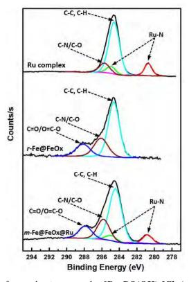
Figure 25. XPS spectra of the free ruthenium complex [Ru-PO(OH)<sub>2</sub>]Cl<sub>2</sub> (top), r-Fe@FeOx NPs (middle) and m-Fe@FeOx@Ru NPs (bottom) in the C1s - Ru 3d region (red and green curves: Ru-N 3d<sub>5/2</sub> and 3d<sub>3/2</sub> signals, respectively; cyan curve: C-C/C-H signal; brown curve: C-N/C-O signal; blue curve: C=O/O=C-O signal).
