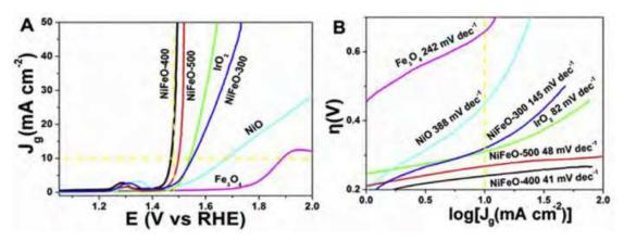
Figure 16. A) the iR-corrected LSV curves of NiFe oxide NCs compared with IrO<sub>2</sub>, NiO, and Fe<sub>3</sub>O<sub>4</sub> in 1M KOH solution at the scan rate of 10 mV/s and B) the corresponding Tafel plots at the current density of  $10 \text{ mA/cm}^2[19]$ .
