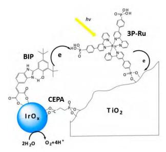
**Figure 8**. Schematic presentation of the electron transfers and water oxidation reaction in the mediator-based, dye sensitized TiO<sub>2</sub> photoanode showing molecular structures of benzimidazole-phenol (BIP) mediator, 3P-Ru dye, and 2-carboxyethyl phosphonic acid (CEPA) anchoring group[51].
