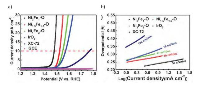
**Figure 6**. a) LSV curves and b) corresponding Tafel plots of  $Ni_2Fe_1$ -O,  $Ni_1SFe_1$ -O,  $Ni_1Fe_2$ -O,  $IrO_2$ , XC-72, and glassy carbon electrode (GCE) in 1M KOH solution at scan rate 5 mV/s[43].
