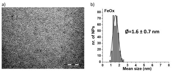
Figure 21. TEM image of a) FeOx NPs (scale bar = 50 nm) and b) corresponding size histogram  $d=1.6\pm0.7$  nm.
