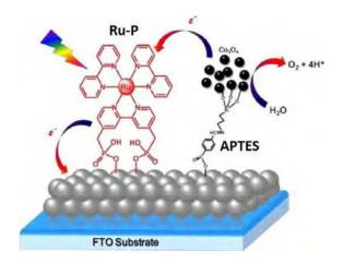
**Figure 10**. Schematic illustration of the  $TiO_2$  electrode (grey balls) co-sensitized by a Ru-polypyridyl complex (RuP) and surface modified  $Co_3O_4$  NPs. reproduced from ref. [53].
