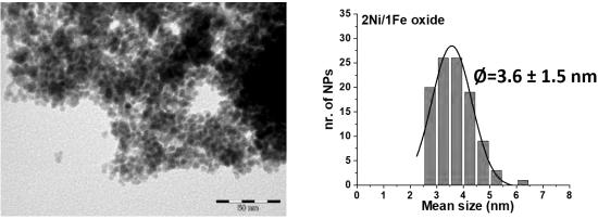
Figure 34. TEM image of a) sample 1Ni/1Fe oxide NPs (scale bar = 50 nm) with b) corresponding size histogram with the average diameter of  $3.1 \pm 1.1$  nm, and TEM image of c) sample 2Ni/1Fe oxide NPs with d) corresponding size histogram with the average diameter of  $3.6 \pm 1.5$  nm.
