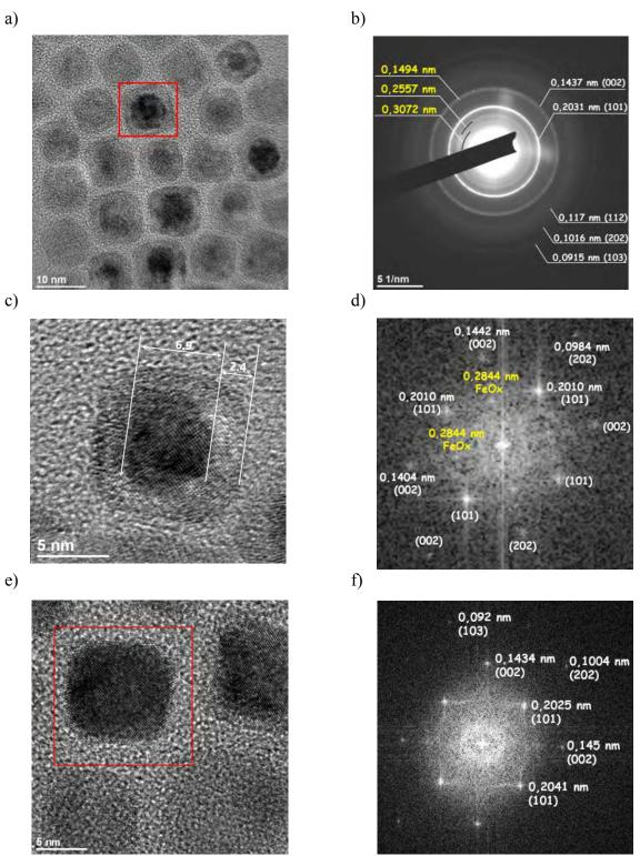
Figure 24. a) HR-TEM of NPs (n-Fe@FeOx NPs), b) selected area electron diffraction pattern, c) typical HR-TEM image of one NP (n-Fe@FeOx NP), d) FFT calculation on the NP highlighted by the red square in a), e) HR-TEM of n-Fe@FeOx NPs, f) FFT calculation on the NP highlighted by the red square in e).
