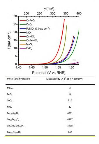
**Figure 4**. Current study – potential curves of different metal oxide thin films deposited on Au substrates in 1M KOH (top) and summary of intrinsic mass activity of various thin film metal oxide/(oxy)hydroxide for OER in 1M KOH at  $\eta$ =350 mV (bottom) [6].
