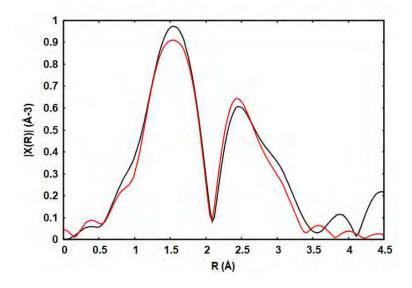
**Figure 35.** Magnitude of the Fourier Transform of function Chi(k), **r-Fe@FeOx NPs** (black line) and best fit achieved (red line)
