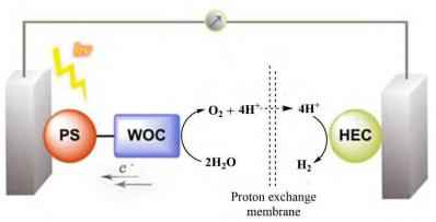
Figure 10. Schematic picture of a molecular assembly for overall H<sub>2</sub>O splitting consisting of a photosensitizer (PS), a water oxidation catalyst (WOC), and a hydrogen evolving catalyst (HEC), for the production of solar fuels, adapt from ref.[21].
