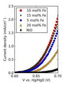
**Figure 6**. Geometric area - normalized polarization (scan rate =  $1 \text{mV.s}^{-1}$ ) data of mixed Ni-Fe oxide catalyst (synthesis by the EISA method) showing the highest activity for 10 at.% Fe. The equilibrium potential for  $O_2$  evolution is approximately 0.308 V vs Hg/HgO[7].
