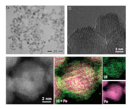
Figure 12. Electron microscopy characterization of FeOx-NiOx core-mixed shell NPs A) TEM image overview of the NPs with an average diameter of  $9.8 \pm 1.6$  nm: B) HR-TEM and HAADF-STEM images displaying a representative NP in A with a crystalline core and a thin amorphous shell; (D) EELS mapping of the NP in C with Ni (green), Fe (pink), and Ni-Fe overlaid maps confirming the core-shell structure[18].
