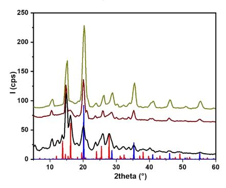
Figure 32. WAXS diagram of n-Fe@FeOx NPs (dark yellow line), a-Fe@FeOx NPs (burgundi line), r-Fe@FeO<sub>x</sub> NPs (black line), in comparison with bcc-Fe (PDF-01071-4648, blue line) and hypothetical maghemite ( $\gamma$ -Fe<sub>2</sub>O<sub>3</sub>) (PDF-01-089-5894, red line).
