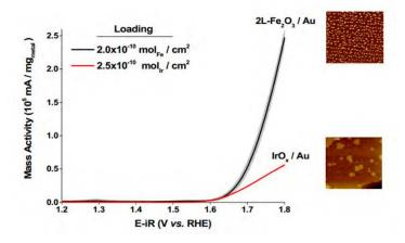
Figure 8. OER voltammograms of 2L-Fe<sub>2</sub>O<sub>3</sub>/Au and ultrathin IrOx/Au catalysts at similar loadings ( $2.0x10^{-10}$  and  $2.5x10^{-10}$  mol metal/cm<sup>2</sup>, respectively). The 2L-Fe<sub>2</sub>O<sub>3</sub>/Au voltammogram represents the average of two independently synthesized samples and the shaded region represents the standard deviation. STM conditions: I = 5 pA, V = 2.0 V; image sizes: 200 nm x = 20
