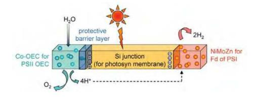
Figure 9. Construction of an artificial leaf[60].
