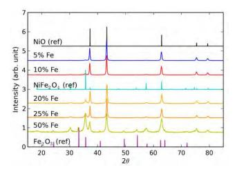
**Figure 7**. XRD patterns of the 5, 10, 20, 25, and 50 at.% Fe mixed samples. Lattice constants for NiO and all mixed Ni-Fe oxides were found to be 4.18 A°, suggesting Fe was not substitutionally incorporated into the NiO lattice[7].
