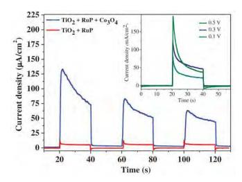
**Figure 11**. The transient current response with 0.3 V vs. Ag/AgCl bias potential for the photoanodes  $TiO_2/RuP/Co_3O_4$ , and  $TiO_2/RuP$ , 1 cm<sup>2</sup> active area in pH=6.8 phosphate buffer solution upon the on-off cycles of illumination (500 W Xe lamp coupled to a 400 nm long-pass filter, 100 mW/cm<sup>2</sup>). Insert: the photocurrent transient for the photoanode ( $TiO_2/RuP/Co_3O_4$ ) under different applied potential[53].
