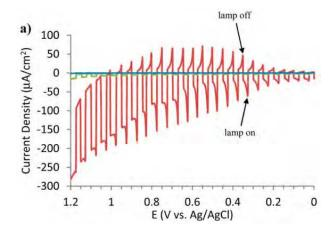
**Figure 6**. Photocurrent transients vs. applied potential for ITO/PMPDI/CoOx (red line), ITO/PMPDI (green line), and bare ITO (Blue line) photoanode in 0.1 M pH 7 KPi buffer, 5mV.s scan rate starting from 0 V (i.e., from right to left) with 5 s light transients[11].
