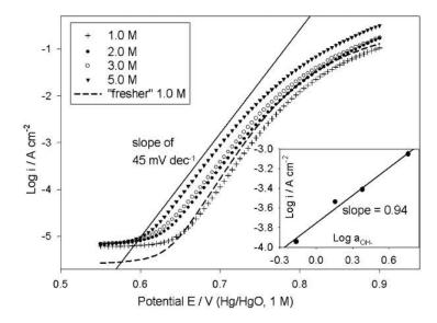
**Figure** OER steady state polarization curves for a pre-reduced Fe various NaOH solutions. The trace denoted as ''fresher 1.0 M" was recorded for earlier reproducibility same electrode in an experiment, before satisfactory with Tafel slope had become established. respect to Inset-reaction order plots constructed from the reproducible polarization data at a potential of E = 0.7 V [4].
