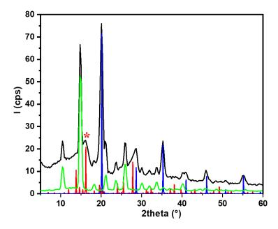
Figure 28. Wide-Angle X-Ray Scattering (WAXS) diagram of a-Fe@FeOx NPs (black solid line), in comparison with reference diagrams of bcc-Fe (PDF-01071-4648, in blue), NH<sub>4</sub>Cl (PDF 96-901-0007, in green), and hypothetical maghemite ( $\gamma$ -Fe<sub>2</sub>O<sub>3</sub>) (PDF-01-089-5894, in red). \*: highlight peak corresponding to maghemite.
