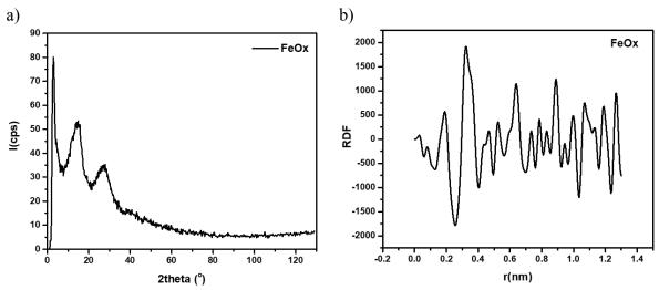
Figure 24. a) WAXS diagram and b) RDF of Fe(0) NPs after oxidation in air for 4 days.
