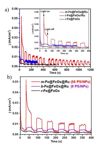
Figure 31. (a) I-t curves recorded on m-Fe@FeOx@Ru NPs (red trace), r-Fe@FeOx//Ru (blue trace) and r-Fe@FeOx NPs (black trace) photoanodes; (b) I-t curves recorded on m-Fe@FeOx@Ru NPs (red trace), b-Fe@FeOx@Ru NPs (purple trace) and r-Fe@FeOx (black trace) photoanodes. Applied potential: 1.0 V vs. RHE. Electrolyte: pH 13 NaOH solution. Incident light power: 100 mW/cm².
