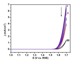
**Figure 50**. Superposition of 50 Cyclic voltammograms (CVs) for FeOx-HMDS NPs in 1M KOH electrolyte. Black arrow emphasizing the decrease in catalytic activity upon consecutive scans.
