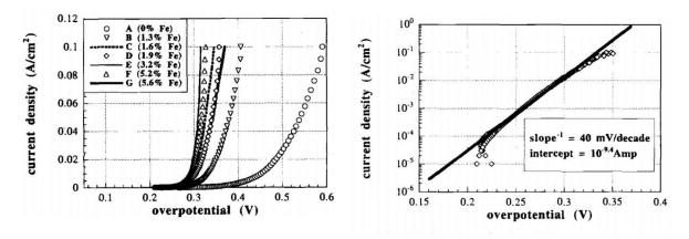
**Figure 5**. a) Steady-state polarization plots of Fe:NiOx anode and b) Tafel plot showing extrapolation to obtain the Tafel slope and exchange current density in 1M KOH[6].
