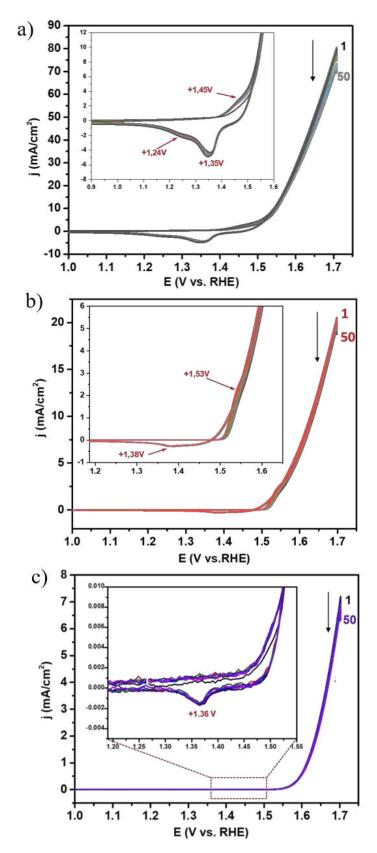
Figure 51. 50 first CVs of a) 2Ni/IFe oxide-APA, b) INi/IFe oxide-APA, c) 1Ni/9Fe oxide-HMDS in KOH 1M, scan rate 5mV/s after activation by LSV
