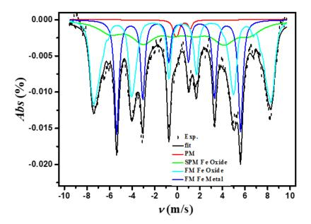
Figure 37. Mössbauer spectrum of r-Fe@FeOx NPs recorded at 80K (experimental data in diamonds), and best fit obtained (solid line) from a combination of iron and iron oxide contributions (see legend on the figure)
