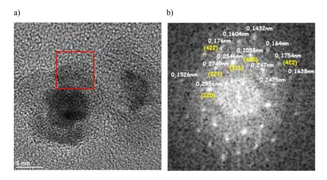
**Figure 30**. a) Typical HR-TEM image of a nanoparticle from **r-Fe@FeOx NPs** sample and b) FFT calculation from the iron oxide layer highlighted by red square.
