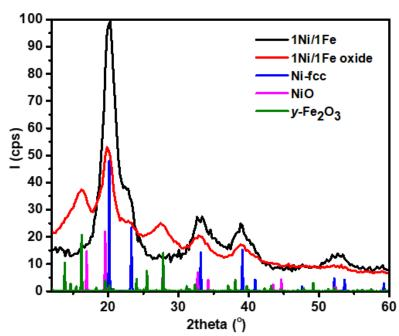
**Figure 37**. WAXS diagram of 1Ni/1Fe NPs before and after air exposure as well as reference fcc-Ni (PDF 04-010-6148), NiO (PDF 00-044-1159), and  $\gamma$ -Fe<sub>2</sub>O<sub>3</sub> (PDF-01-089-5894) diagrams.
