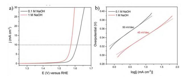
**Figure 15.** a) Rotating disk electrode (RDE) voltammogram with iR compensation and d) corresponding Tafel plots obtained with the  $\gamma$ -Fe<sub>2</sub>O<sub>3</sub>/CNT electrode in 0.1 M (black lines) and 1.0 M (red lines) NaOH. Potential scan rate of 5mV/s and rotation of 1600 rpm[14].
