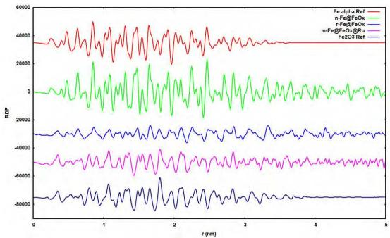
Figure 23. Comparison between RDF of, from top to bottom, model bcc-Fe NPs, n-Fe@FeOx NPs, r-Fe@FeOx NPs, and model γ-Fe<sub>2</sub>O<sub>3</sub> NPs showing the evolution from a nanomaterial with a high bcc Fe content to one with a high crystalline maghemite content.
