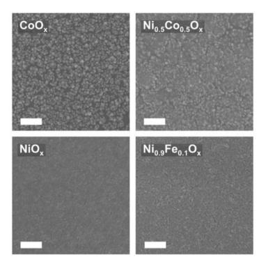
**Figure 10**. SEM image of selected thin films ( $CoO_x$ ,  $Ni_{0.5}Co_{0.5}O_x$ ,  $NiO_x$  and  $Ni_{0.9}Fe_{0.1}O_x$ ) deposited on a Si electrode by the solution deposition method. Scale bars are 100 nm[2].
