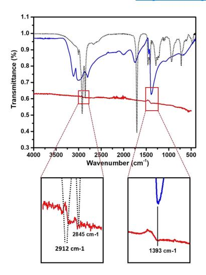
Figure 22. ATR-IR spectrum of n-Fe@FeOx NPs (red solid line) in comparison with oleic acid (black dotted line) and NH<sub>4</sub>Cl (blue solid line).
