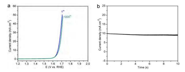
**Figure 10**. a) Polarization curves for  $\alpha$ -Fe<sub>2</sub>O<sub>3</sub> NA/CC in 0.1 M KOH initially and after 1000 CV scanning between +1.2 and +2.0 V (vs. RHE). (b) Time-dependent current density curve for  $\alpha$ -Fe<sub>2</sub>O<sub>3</sub> NA/CC in 0.1 M KOH at an overpotential of 420 mV over a period of 10 h[12].
