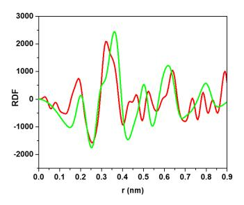
**Figure 26**. Radial distribution function of FeOx-HMDS (red line) compared with a simple model of hematite with 30 atoms (green line)
