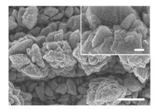
**Figure 6**. SEM images of as-prepared c-Fe<sub>2</sub>O<sub>3</sub>. The insert shows the surface morphology at higher magnification. Scale bar:  $1\mu m$ , insert 100 nm [7].
