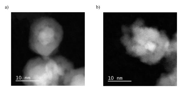
Figure 20. HR-HAADF-STEM images of a) b-Fe@FeOx@Ru NPs and b) m-Fe@FeOx@Ru NPs.
