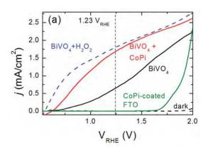
**Figure 1**. a) Cross section scanning electron microscope image of a 30 nm thick Co-Pi modified  $BiVO_4$  photoanode and b) AM 1.5 photocurrent vs voltage curve for a  $BiVO_4$  photoelectrode and a Co-Pi modified  $BiVO_4$  photoelectrode recorded at a scan rate of 50 mV/s. The reference curves for Co-Pi coated FTO confirms the true photovoltaic nature of the photocurrents in  $BiVO_4$  and rules out that they are caused by photoconductivity effects[43].
