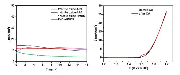
Figure 47. a) CA assessment of 2Ni/1Fe oxide-APA NPs (red line), 1Ni/1Fe oxide-APA NPs(black line), 1Ni/9Fe oxide-HMDS NPs(purple line), and FeOx-HMDS NPs (green line) at j=10 mA/cm² in 1M KOH; b) LSV curves of sample 2Ni/1Fe oxide- APA NPs before and after the CA test.
