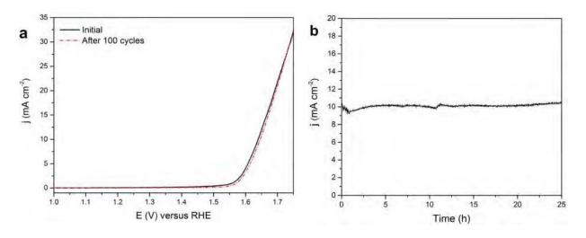
Figure 16. Stability test of the  $\gamma$ -Fe<sub>2</sub>O<sub>3</sub>/CNT catalyst for OER a) the polarization curves of  $\gamma$ -Fe<sub>2</sub>O<sub>3</sub>/CNT before the cycling durability test (black solid line) and after 100 cycles (red dash dot line) between the potential of 1 and 1.75 V vs. RHE. Potential scan rate of 50 mV/s b) time dependence of the current density obtained at a static potential of ~1.64 V vs. RHE in 0.1 M NaOH[14].
