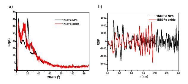
Figure 29. a) WAXS diagrams and b) RDFs of 1Ni/9Fe oxide-HMDS NPs before and after oxidation in air for 4 days.
