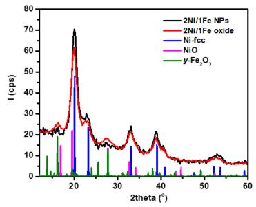
**Figure 38**. WAXS diagram of 2Ni/1Fe NPs before and after air exposure as well as reference fcc-Ni (PDF 04-010-6148), NiO (PDF 00-044-1159), and  $\gamma$ -Fe<sub>2</sub>O<sub>3</sub> (PDF-01-089-5894) diagrams.
