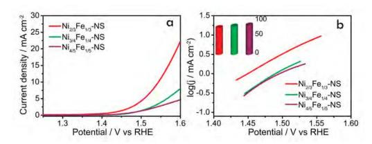
**Figure 4**. a) iR- corrected polarization curves and b) Tafel slopes of  $Ni_{2/3}Fe_{1/3}$ -NS,  $Ni_{3/4}Fe_{1/4}$ -NS, and  $Ni_{4/5}Fe_{1/5}$ -NS (inset: histogram of corresponding Tafel slopes)[16].
