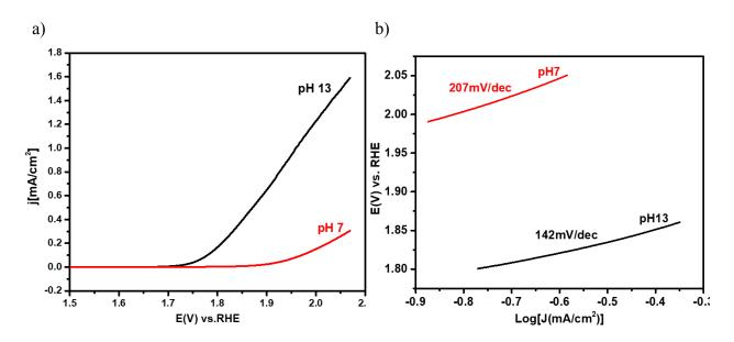
Figure 48. a) Polarization curves of a r-Fe@FeOx NPs electrode recorded in pH 7(red line) and pH 13 (black line) electrolyte solutions, potential scan rate was 5 mV/s. b) Tafel slope of r-Fe@FeOx NPs electrode in pH 7(red line) and pH 13 (black line).
