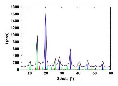
Figure 25. Wide-Angle X-Ray Scattering (WAXS) diagram of n-Fe@FeOx NPs (black solid line) in comparison with reference diagrams of bcc-Fe (PDF-01071-4648, in blue), NH<sub>4</sub>Cl (PDF 96-901-0007, in green) and hypothetical maghemite γ-Fe<sub>2</sub>O<sub>3</sub> (PDF-01-089-5894, in red).
