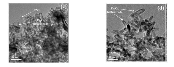
Figure 12. TEM images of  $\alpha$ -Fe<sub>2</sub>O<sub>3</sub>/CNT composite[13].
