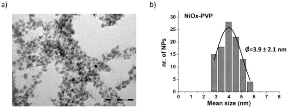
Figure 20. TEM image of a) NiOx-PVP NPs (scale bar = 50 nm) and b) corresponding size histogram  $d=3.9\pm2.1$  nm.
