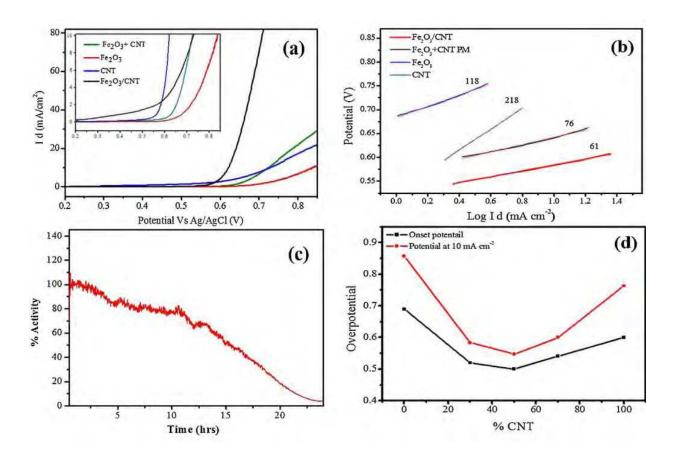
Figure 13. Comparison between the electrocatalytic activities of  $\alpha$ -Fe<sub>2</sub>O<sub>3</sub> and  $\alpha$ -Fe<sub>2</sub>O<sub>3</sub>/CNT composite (a) polarization curve from the catalyst deposited on glassy carbon electrode, (b) corresponding Tafel plots, (c) potentiostatic analysis at a constant potential of 600 mV V vs. Ag/AgCl electrode, (d) effect of CNT loading on the onset potential and potential at a current density of 10 mA/cm<sup>2</sup>[13].
