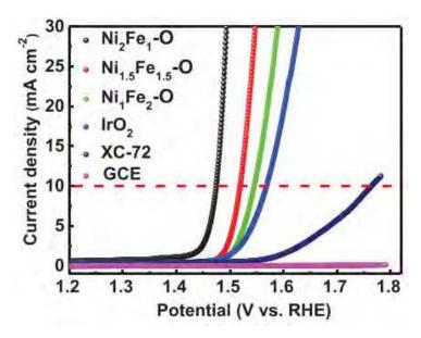
Figure 5. LSV curves of  $Ni_2Fe_1$ -O,  $Ni_1.5Fe_1.5$ -O,  $Ni_1Fe_2$ -O,  $IrO_2$ , XC-72, and glassy carbon electrode (GCE) in 1M KOH solution at scan rate 5 mV/s[43].
