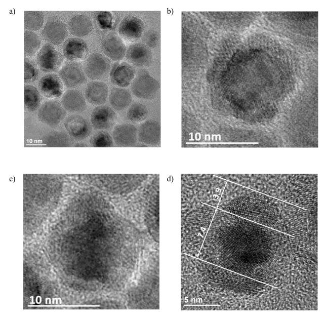
Figure 29. Typical HR-TEM images of nanoparticles from the r-Fe@FeOx NPs sample.
