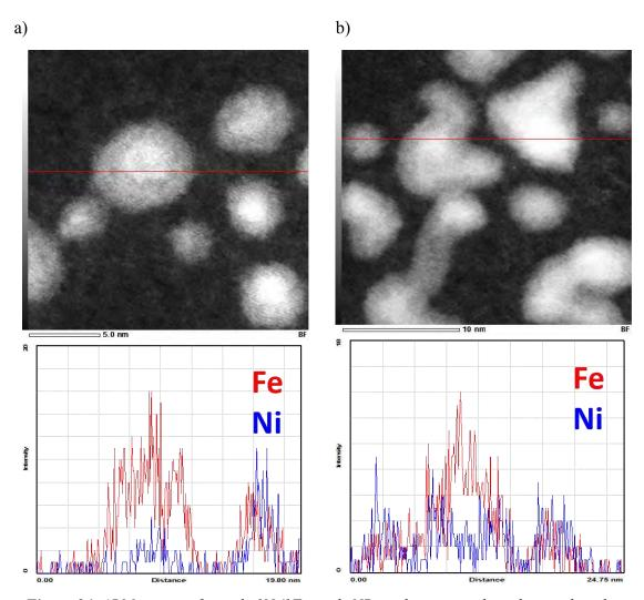
Figure 36. ARM images of sample 1Ni/1Fe oxide NPs and corresponding elemental analysis
