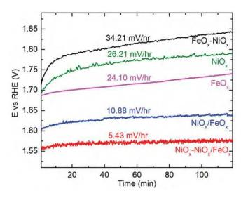
**Figure 14.** CP of the nanocatalyst obtained in 1M KOH at a current density of 10 mA/cm<sup>2</sup> for 2 h: NiOx-NiOx/FeOx core-mixed shell (red line), NiOx/FeOx alloy (blue), FeOx-NiOx core-shell (black), FeOx (pink), and NiOx (green)[18].
