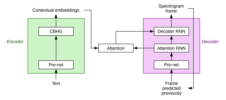
Figure 2.6 – The architecture of the first Tacotron model, introduced by (Wang, Skerry-Ryan, et al. 2017)
