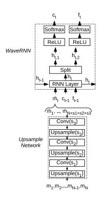
Figure 4.3 – Architecture of the neural vocoder.
