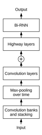
Figure 2.7 – The architecture of the CBHG module, reproduced from (Wang, Skerry-Ryan, et al. 2017)
