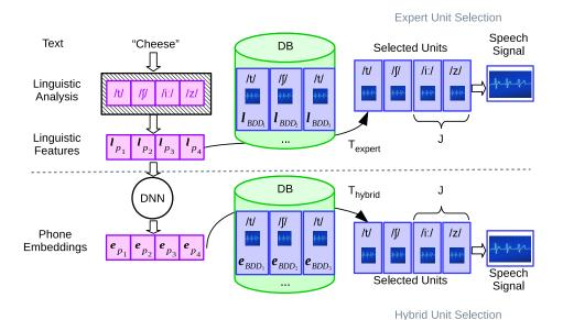
Figure 3.1 – Representation of expert (top of the figure) and hybrid (bottom of the figure) unit selection.  $l_{p,i}$  and  $l_{BD,i}$  refers to the linguistic feature vector of the *i*-th unit of a sentence or in the speech database.  $e_{p,i}$  and  $l_{BD,i}$  refers to the corresponding phone embeddings.  $T_{expert}$  is the expert target cost,  $T_{hybrid}$  is the hybrid target cost, and J is the join cost.
