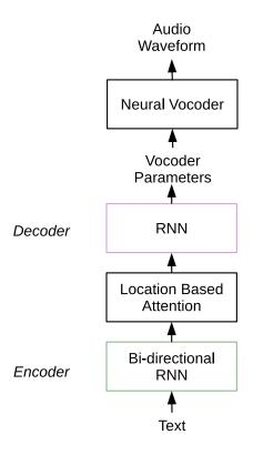
Figure 2.5 – Architecture of the Char2Wav TTS system.
