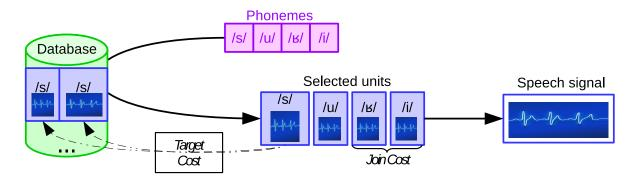
Figure 1.4 – Process to synthesize the sequence of phonemes /suʁi/ using unit selection.
