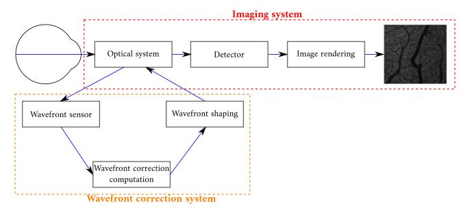
**Figure 1.19** – Sensor based hardware AO (HAO) for correction of aberrations [72]. This is divided between an imaging part and a wavefront correction part. The imaging system aims at producing an image while the wavefront correction system changes the shape of the wavefront hardwarewise. The arrows correspond to the path of the signal containing the information.
