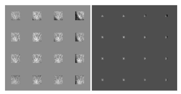
Figure 3.12 – Example of cropped sub-images and corresponding cropped correlation matrices, for  $4 \times 4$  sub-apertures. Here all the sub-images on the right column show a limiting aperture, which spoils the correlation: the corresponding peaks in the correlation matrices are barely or even not visible.
