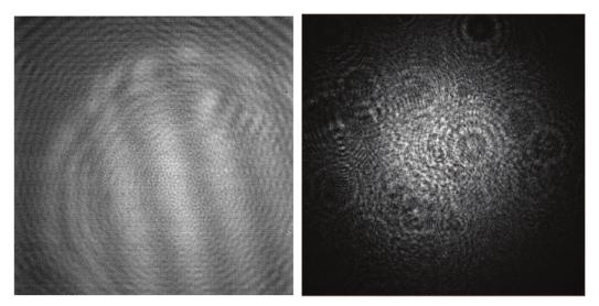
**Figure 2.4** – Interferograms of off-axis FF-SSOCT (left) and laser Doppler imaging (right). The off-axis configuration is well-visible with the delimitation of the smallest diameter beam on the first image.
