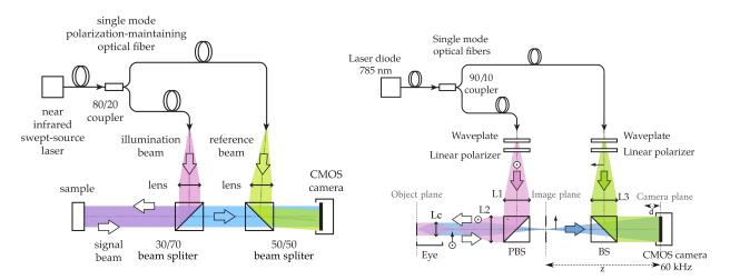
**Figure 2.1** – Schemes of the holographic off-axis OCT (first image) and in-line laser Doppler (second image) setups. In both cases, the reference wave from the source interferes with the object wave which has been reflected on the sample.
