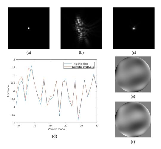
Figure 3.6 – Estimation of the phase for a point source, with a Shack-Hartmann using  $10 \times 10$  subapertures. (a) Source. (b) Aberrated PSF. (c) Corrected PSF. (d) Amplitudes of the Zernike coefficients of the added phase in radians (blue) vs estimated amplitudes (orange). (e) Added phase shape. (f) Estimated phase shape.
