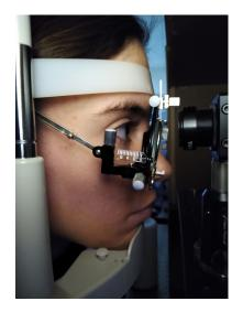
**Figure 3.13** – Photo of the verification experiment. Astigmatic glasses are placed and adjusted in front of the emmetropic eyes using holders.
