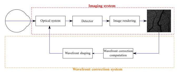
Figure 1.21 – Sensorless AO (SAO) for correction of aberrations [72]. It is very similar to the HAO (fig. 1.19), except the wavefront sensor has been removed. Instead, the correction is based on the image. The compensation to add to the wave is calculated and applied thanks to a hardware corrector.
