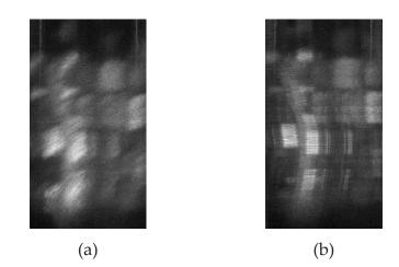
**Figure 2.11** – Profile image of glass beads of 1.5 mm of diameter, before (a) and after (b) rescaling of the acquisitions.
