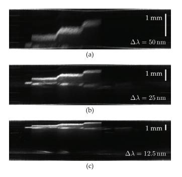
Figure 2.8 – Axial range  $\Delta z$  for a wavelength tuning range  $\Delta \lambda$  of 50 nm (a), 25 nm (b), and 12.5 nm (c). The sample is composed of three scales of tape layers. Each scale is  $\sim 313 \,\mu\text{m}$  height, which was measured with a numerical calliper and confirmed by full-field OCT. The axial field of view  $\Delta z$  of 1.8 mm (a), 3.7 mm (b), and 7.3 mm (c) is in agreement with the theoretical value from Eq. 2.24 for N = 256. Axial scalebar : 1 mm.
