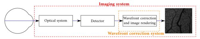
Figure 1.22 – Computational AO (CAO) for correction of aberrations [72]. The light reflected by the retina is sent through the optical system and captured by a sensor. The correction is calculated from this signal and directly applied to produce a corrected image.
