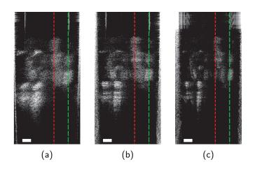
Figure 2.16 – Axial motion compensation in swept-source holographic OCT of glass beads rolled in a tape layer. The registered holograms are slices in the  $(x, \omega)$  plane, for the y-cut in fig. 2.17. Figures represent the sample: (a) without any correction, (b) with interferogram rescaling (eq. (2.16)), and (c) with interferogram rescaling and axial motion compensation. The white scale bars indicate 0.2 mm.
