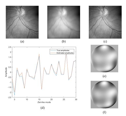
Figure 3.7 – Estimation of the phase for an extended object, with a Shack-Hartmann using  $10 \times 10$  subapertures. (a) Image without aberration. (b) Aberrated image. (c) Corrected image. (d) Amplitudes of the Zernike coefficients of the added phase in radians (blue) vs estimated amplitudes (orange). (e) Added phase shape. (f) Estimated phase shape.
