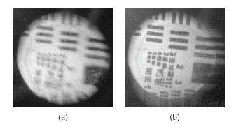
FIG. 4: illustration of chromatic compensation by interferogram resampling. Hologram rendering without interpolation in Vizualization 1.
