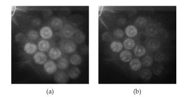
Figure 2.10 - En-face image of glass beads of 1.5 mm of diameter, before (a) and after (b) rescaling of the acquisitions.
