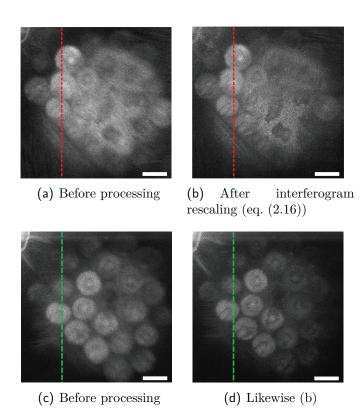
Figure 2.17 – (a,b) En-face (x, y) images of glass beads for the first red z-cut in fig. 2.16, and (c,d) for the second green z-cut in fig. 2.16. The white scale bars indicate 1.5 mm.
