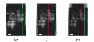
Fig. 3: Axial motion compensation in swept-source holographic OCT of glass beads rolled in a tape layer. The registered holograms are slices in the  $(x, \omega)$  plane, for the ycut in Fig. 4. Figures represent the sample: (a) without any correction, (b) with interferogram rescaling (Eq. (2)), and (c) with interferogram rescaling and axial motion compensation (Section 3.2). The white scale bars indicate 0.2 mm.
