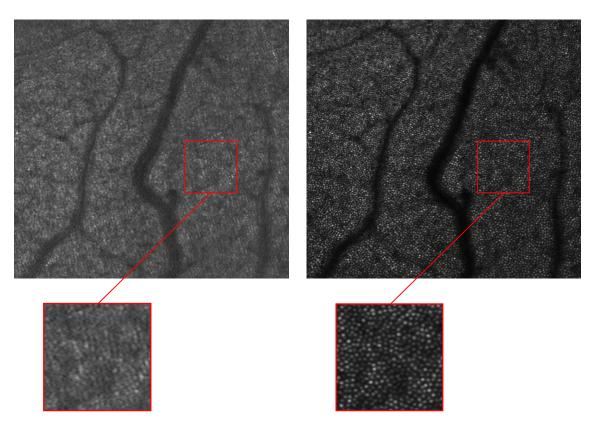
**Figure 1.18** – Images recorded with the PSI AO-SLO device of retina vessels and photoreceptors [71]. Adaptive optics has only been used on the second image. It has significantly improved the resolution of photoreceptors.
