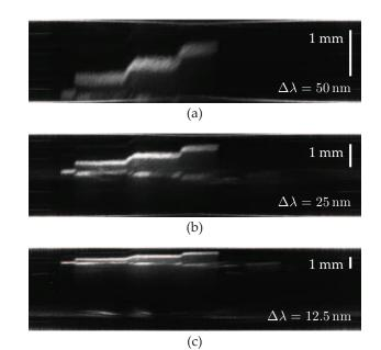
FIG. 2: Axial range  $\Delta z$  vs. wavelength tuning range  $\Delta \lambda$  of 50 nm (a), 25 nm (b), and 12.5 nm (c). The height difference between adjacent scales is ~ 313  $\mu$ m, which was measured by full-field OCT. The axial field of view  $\Delta z$  of 1.8 mm (a), 3.7 mm (b), and 7.3 mm (c) is in agreement with the theoretical value from Eq. 3 for  $N_z = 256$ . Axial scalebar : 1 mm.
