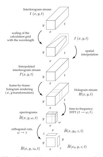
FIG. 3: Flowchart of the main data processing steps. Each interferogram I from the input data stream is rescaled by linear interpolation to I' to compensate for chromatic distortion. Holograms H are calculated by Fresnel transformation from rescaled interferograms I'. Temporal short-time Fourier transforms at each pixel location (x, y) turn holograms H into spectrograms  $\tilde{H}$ . Orthogonal cuts of the magnitude of each spectrogram  $|\tilde{H}|$  are displayed at video rate.
