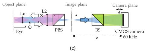
Figure 2.2 – Zooms on the pink optical path from reference to retina (a), green optical path from reference to camera (b), and blue optical path from retina to camera (c). The pink optical path includes L1, L2 and Lc lenses. The green optical path includes L3 lens. The blue optical path includes Lc and L2 lenses.
