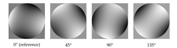
Figure 3.18 – Estimated shape of the wavefront for different orientations of the astigmatism.
