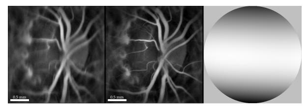
Figure 3.17 – Correction of a laser Doppler image of the model retina, where 6-diopter vertical astigmatism has been added. The first figure represents the image before aberration compensation, while the second one represents the corrected image. The third figure illustrates the shape of the wavefront.
