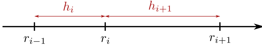
Figure 4.2: Sketch of the discretisation of a 1-D domain with a variable discretisation step.
