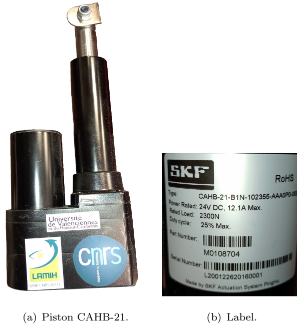
FIGURE 2.2: Linear piston and its label.
