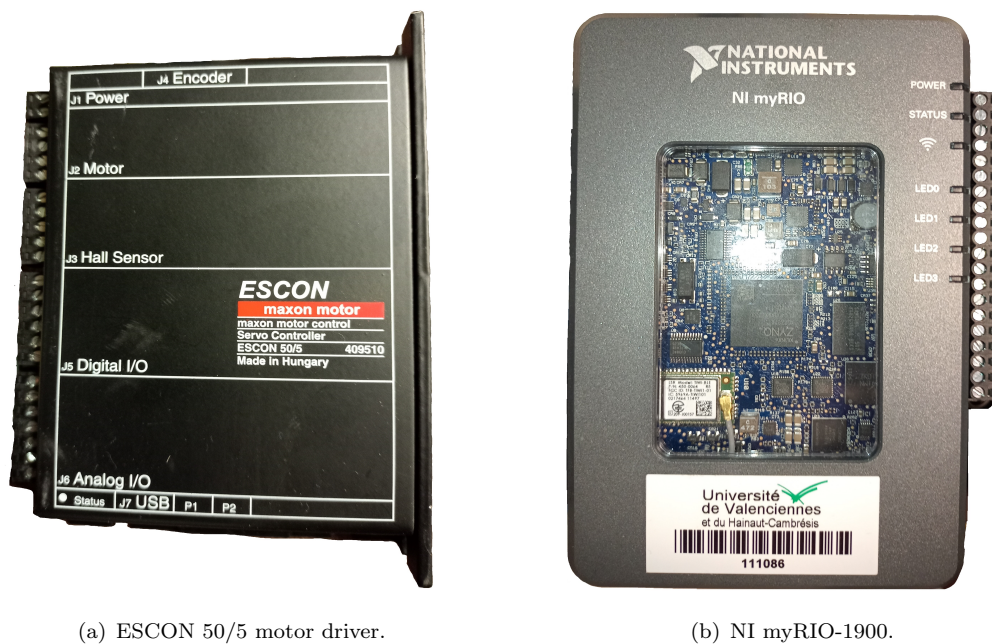
FIGURE 2.4: ESCON 50/5 motor driver and myRIO devices.
