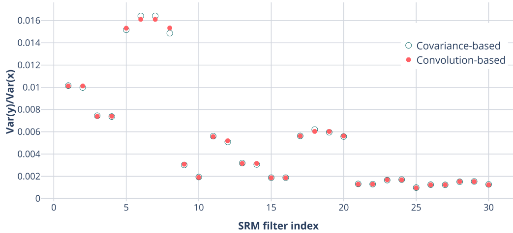
Fig. 4.1.: The value of \text{Var}(y)/\text{Var}(x) for each of the 30 SRM filters obtained by using the covariance-based method of Eq. (4.3) and the convolution-based method.
